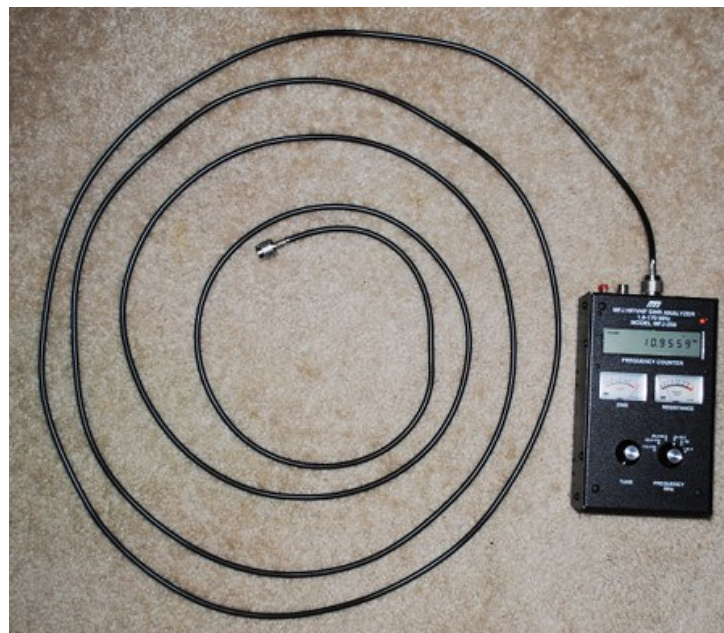
Piece of RG58U attached to MFJ-259
