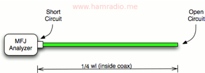
Testing a Quarter Wavelength of Transmission Line
