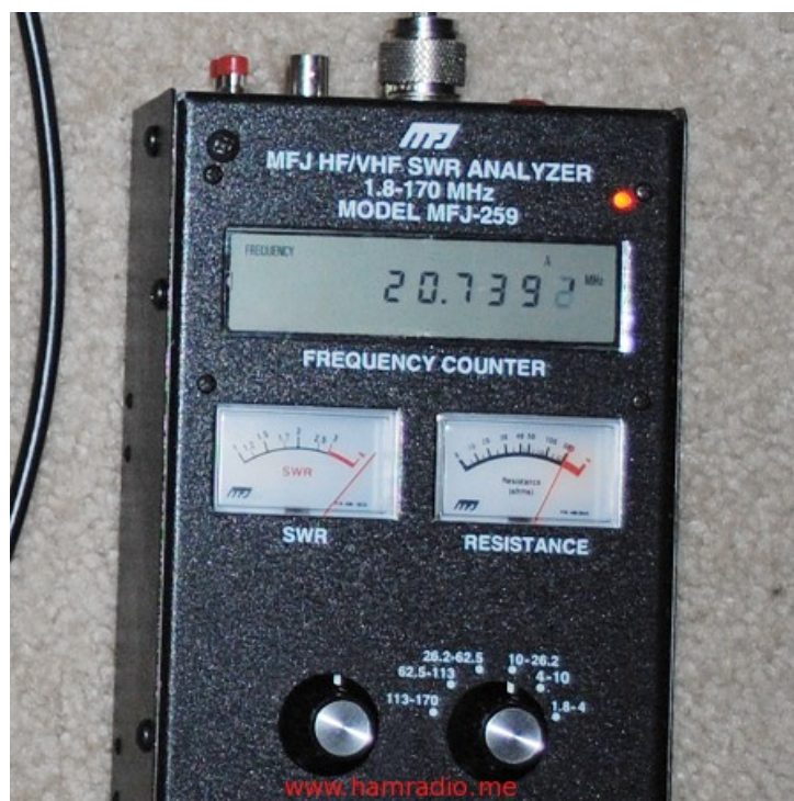
Adjusting MFJ for Maximum Impedance
