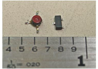
device in the circuit. The PMBFJ176 has an IDSS range of 2 to 35 mA. This is quite a spread so if one doesn't seem to work, try another one. I tried the -174 and -175 models and they didn't seem to work right. This FET is also made by Fairchild and is available from Digi-Key for about 49 cents each.
