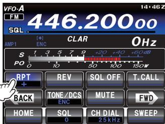
5. Touch **[FWD]** to switch the display screen, and then touch **[TONE]**. Rotate the **MULTI** knob to select the desired CTCSS Tone to be used. A total of 50 standard CTCSS tones are provided (see the CTCSS Tone Chart).
