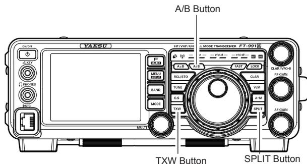
During Split operation, the VFO-A register will be used for reception, while the VFO-B register will be used for transmission. If you press the **SPLIT** button once more, Split operation will be cancelled.
