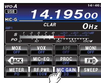
*In the AM mode*, touch [**MIC GAIN**] and then adjust the **MULTI** knob so that the ALC meter does not deflect on voice peaks.
