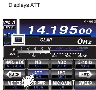
2. To restore full signal strength through the Attenuator circuit, touch [ATT] on the LCD to return the ATT display to the “OFF” position.
