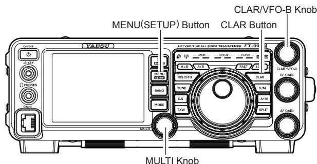
7. Rotate the **CLAR/VFO-B** knob to set the desired transmitter offset. A maximum split of  $\pm 9.999$  kHz may be set.
