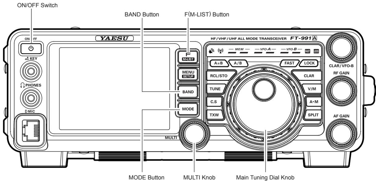
1. Press the **BAND** button to show the band list, and then touch a band key corresponding to the Amateur band on which you wish to operate. Press the **BAND** button again, to close the band list screen.
