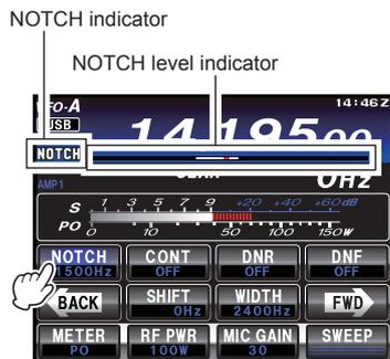
3. Rotate the **MULTI** knob to adjust the “null” position of the Notch filter.
