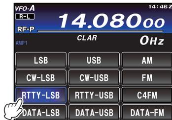
3. Press the **MENU(SETUP)** button. The Menu list will appear in the display. Rotate the **MULTI** knob to select Menu item “060 PC KEYING”. Touch [**SELECT**] on the LCD, then rotate the **MULTI** knob to set this Menu item to “RTS” or “DTR”. Press the **MENU(SETUP)** button or touch [**BACK**] on the LCD to exit to normal operation.
