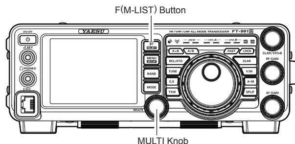
4. Start sending and rotate the **MULTI** knob to adjust the hang time, as you prefer for comfortable operation.
