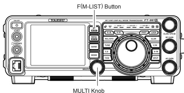
3. Press and hold in the microphone **UP** or **DWN** button for one second, or press the **F(M-LIST)** button followed by **[SCAN]** to start scanning in the specified direction on the VFO frequency.
