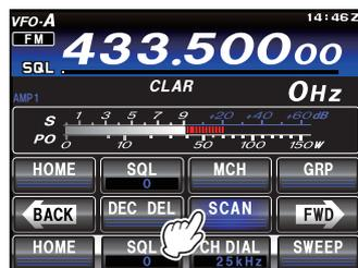
4. If the scanner halts on an incoming signal, the decimal point between the “MHz” and “kHz” digits of the frequency display will blink.
