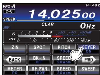
4. Touch **[SPEED]** on the LCD, then rotate the **MULTI** knob to set the desired sending speed (4 - 60 WPM).
