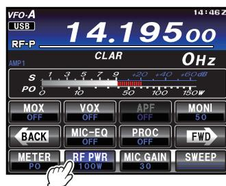
5. Adjust the microphone amplifier gain to match the microphone and your voice level: Touch [**METER**] on the LCD repeatedly to select the “ALC”. Press and hold the **PTT** switch, and speak into the microphone in a normal voice level.
