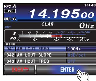
6. Press the **MENU** button or touch **[BACK]** on the LCD to exit to normal operation.
