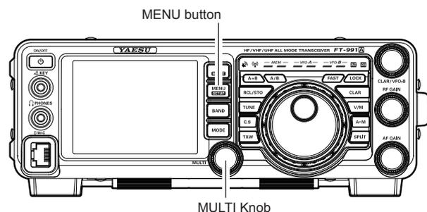
4. Rotate the **MULTI** knob to the point where the offending noise is best reduced or eliminated.
