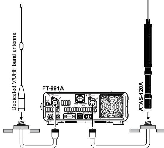
When using an antenna duplexer, the ANT terminal of the **ATAS-120A** and the HF/50 MHz ANT terminal of the **FT-991A** must be connected in series and also insulated from the grounding in order to supply the control voltage for the **ATAS-120A**.
