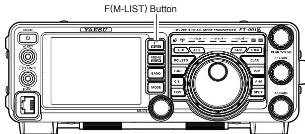
2. If desired, the Noise Blanker level may be adjusted via Menu item “025 NB LEVEL” to the point where the offending noise is best reduced or eliminated. See box below for details.
