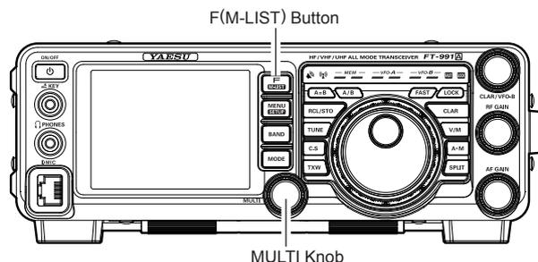
3. Rotate the **MULTI** knob to set the sound volume to a comfortable level.
