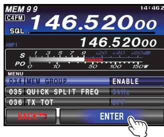
5. Press the **MENU(SETUP)** button or **[BACK]** on the LCD to exit. Operation will now be restricted to the six Memory Groups.
