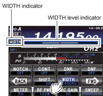
2. Rotate the **MULTI** knob counter-clockwise to narrow the bandwidth and reduce interference.
