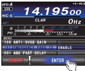
5. Press the **MENU(SETUP)** button or **[BACK]** on the LCD to exit to normal operation. Emergency communication on this spot frequency is now possible.
