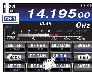
2. Touch **[CH DIAL]** to select the desired frequency step. Touching **[CH DIAL]** switches the frequency as follows.
