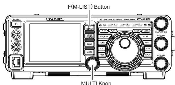
3. Rotate the **MULTI** knob to choose one of 15 algorithms that best reduces the noise level.
