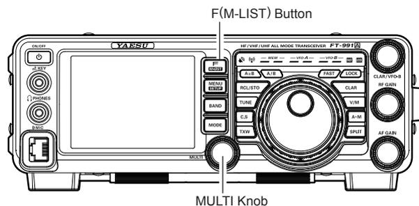
3. Press the **F(M-LIST)** button, then touch [**PROC**] to display the PROC level (from 1 to 100), confirming that the Speech Processor is engaged.
