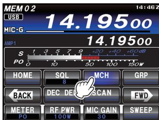
8. Rotate the **MULTI** knob to select the emergency channel (“EMG”), which is found between channels “5-10” and “01ch”).
