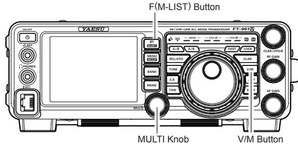
3. Press and hold in the microphone **UP** or **DWN** button for one second, or press the **F(M-LIST)** button followed by **[SCAN]** to start scanning in the specified direction.
