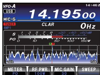
3. Press and hold in the **TUNE** button for one second to begin automatic tuning. The transmitter will be engaged, and the “**TUNER**” icon will blink while tuning is in progress. When the optimum tuning point has been reached, the radio will return to receive, and the “**TUNER**” icon will again glow steadily (instead of blinking).
