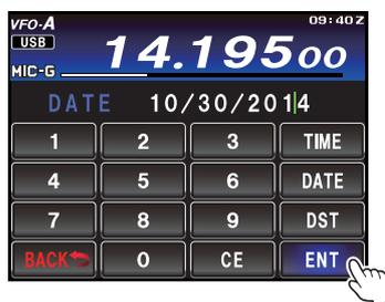
6. Touch **[BACK]** on the LCD to return to the setup mode display.
