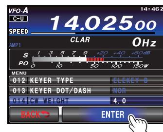
5. Press the **MENU(SETUP)** button or touch [**BACK**] on the LCD to exit to normal operation.
