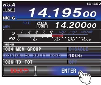
5. Press the **MENU(SETUP)** button or touch [BACK] on the LCD to exit to normal operation.
