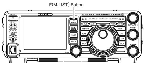
To disable the Digital NOTCH Filter, just repeat the above procedure, touching **[DNF]** on the LCD to choose “OFF”. The “DNF” will turn off, confirming that the Digital NOTCH Filter is not active.
