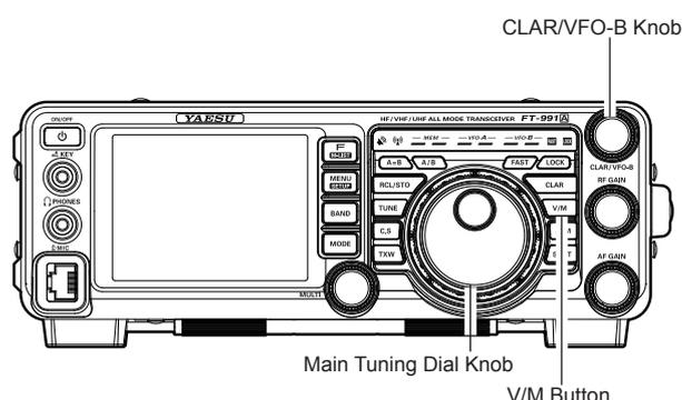
3. Memory channels (“5-01” through “5-10”) are pre-programmed, at the factory, with the permitted frequencies in the 5 MHz band, and the USB or CW mode is automatically selected on these channels.
