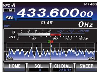
6. Press the **A▶M** button. Make sure that the memory channel storing the receive frequency is selected.
