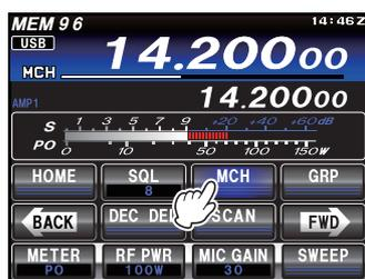
3. Touch **[MCH]** on the LCD, and then rotate the **MULTI** knob to select the desired memory channel.
