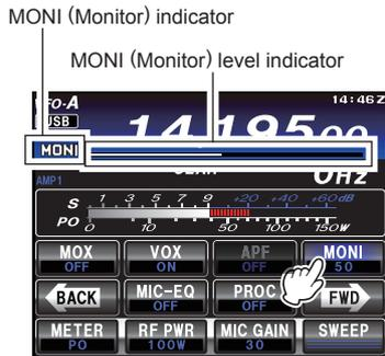
3. During transmission, rotate the **MULTI** knob to adjust the audio level in the Headphones or speaker. Clockwise rotation of this knob will increase the volume level.
