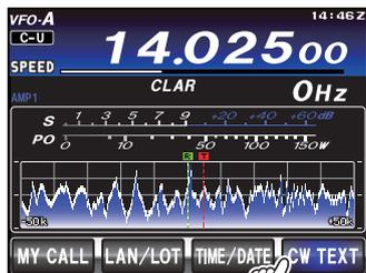
3. Rotate the **MULTI** knob to select the CW TEXT you want to input, then touch [**EDIT**]. The text input screen will appear.
