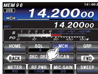
5. Rotate the **MULTI** knob to select the desired Memory Channel within the Selected Memory Group.
