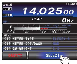
4. When your adjustments are complete, touch [**ENTER**] on the LCD to save the new setting.
