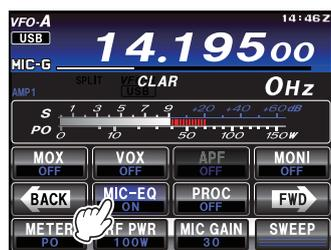
To adjust the Parametric Microphone Equalizer with the speech processor engaged, press the **F(M-LIST)** button, then touch **[PROC]** to select “ON”.
