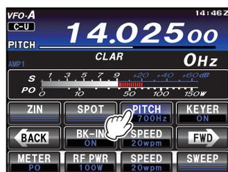
2. Rotate the **MULTI** knob to adjust the PITCH (300 Hz to 1,050 Hz).
