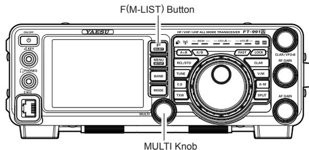
2. Rotate the **MULTI** knob to the left or right to reduce interfering signals.
