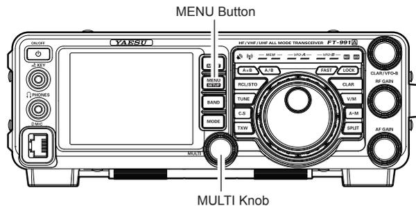
4. Rotate the **MULTI** knob to adjust the receiver audio response as desired.
