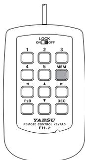
5. Touch **[CH1]** through **[CH5]** on the LCD or press any of the **FH-2** keys numbered **[1]** through **[5]** to begin the memory storage process, and the “REC” icon will glow steadily.
