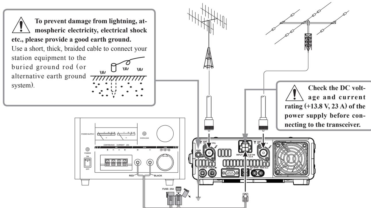
We recommend the use of the **FP-1030A** (USA market only) AC Power Supply. Other models of power supplies may be used with the **FT-991A**, but the 13.8 VDC input voltage, 23 Ampere current capability, and DC cable polarity guidelines described above must be strictly followed.
