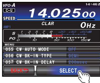
4. When the adjustments are complete, touch [**ENTER**] on the LCD to save the new setting.
