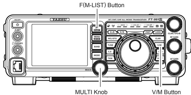
3. Rotate the **MULTI** knob to select the memory channel.
