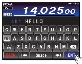
5. Repeat step 4 to program the remaining letters, numbers, or symbols of the desired text. 12 characters may be used in the creation of a text. Use [**←**] and [**→**] on the LCD to set the cursor position and [**✕**] on the LCD to erase a letter at the left of the cursor.
