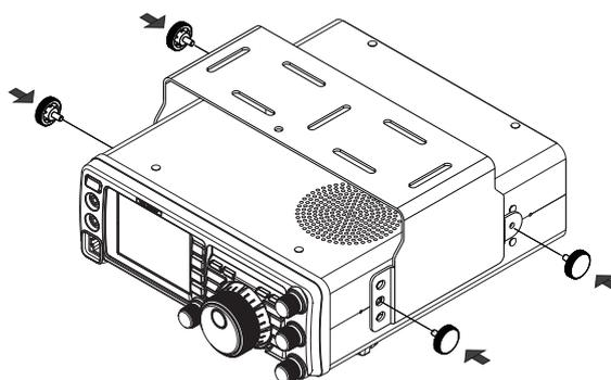
The viewing angle of the transceiver may be adjusted by changing the location of the front mounting screws.
