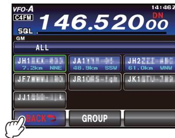
Up to 24 stations operating with the GM function within the sphere of communications will be listed on the TFT display.
