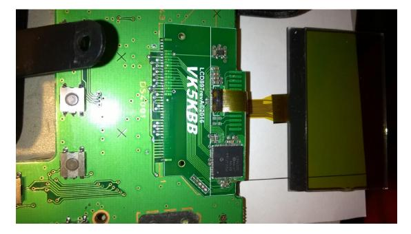
While it is soaking you can fit the new LCD PCB assembly.
