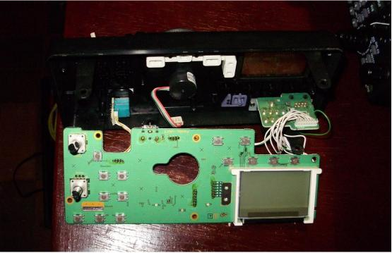
There is no need to remove the frequency dial but the other knobs must be pulled off. A soft plastic pry like a guitar pick is suitable.
