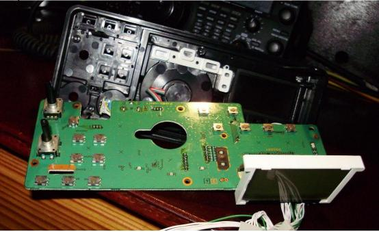
Revealing the solder joint and the flex-ribbon cable.
