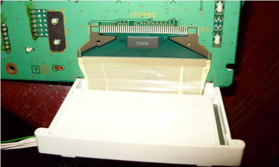
I normally cut the flex with old scissors to remove the LCD and light-pipe assembly. One can also gently roll the flex up off the PCB as it is held with double sided adhesive.
