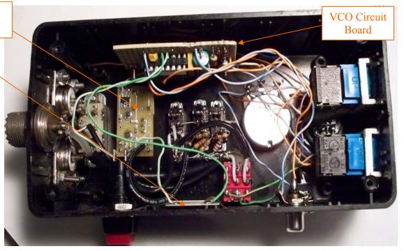
The schematic for this unit is included at the end of this document. The active attenuator is an "offset attenuator" PCB kit from Marvin Johnson, KE6HTS. The 74HC4046 VCO is powered by the 8V from the mic jack as well, with 4 series diodes providing a voltage drop to operate the VCO in a safe voltage region. The S meter voltage drives the VCO, and the output of the VCO drives the Piezo speaker.
