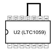
Connect pins 9 & 11 as shown to the left. Remember that pin 9 is not to be inserted into the circuit board!
