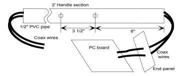
99. Solder the coax to the narrow antenna mounting PC boards. Pay special attention to the orientation of the boards, Note that the larger antenna mounting holes face outwards, lining up with the pre-drilled holes in the PVC pipe. Use the same soldering technique that was used
