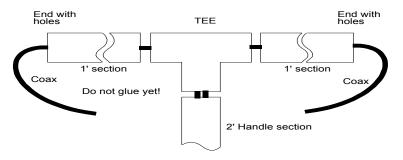
98. Thread the coax through the 1 foot PVC pipe sections. Have the ends with the pre-drilled holes facing away from the TEE.
