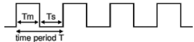
555 astable output, a square wave ( T_m and T_s may be different)
