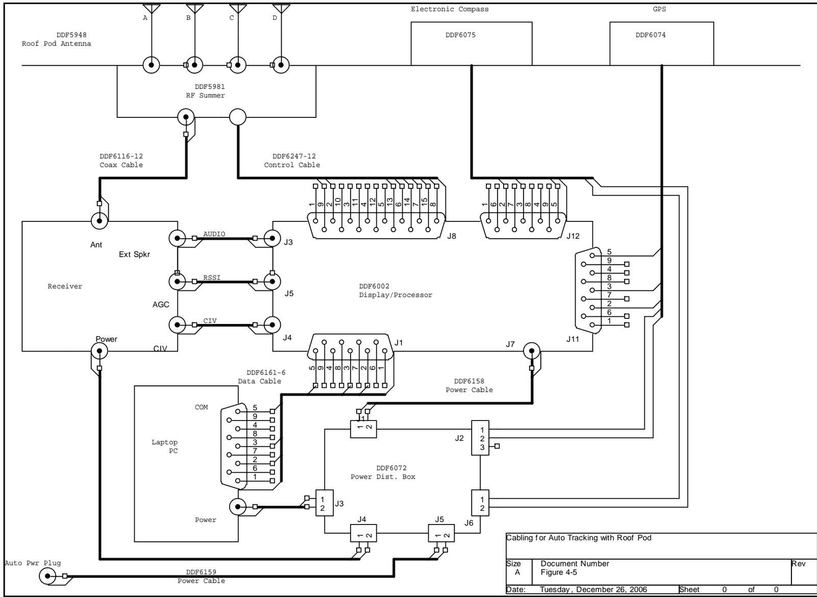
Cabling for Auto Tracking with Roof Pod
