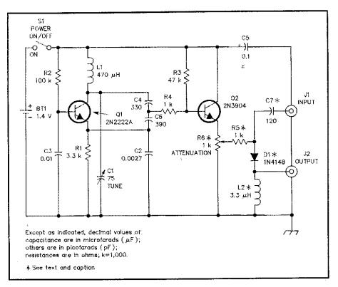
Fig 1—Schematic of the active attenuator. Resistors are ¼-W, 5%-tolerance carboncomposition or film. R6 is mounted on the wall of the metal enclosure. (The author used a slide control at R6; a rotary control is also suitable.) R5, C7, D1 and L2 are connected between the input/output connectors, ground and R6.
