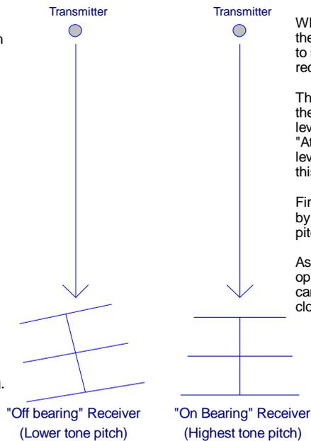
When heading towards the transmitter the pitch of the signal tone will continue to increase to a point just before the receiver saturates.
