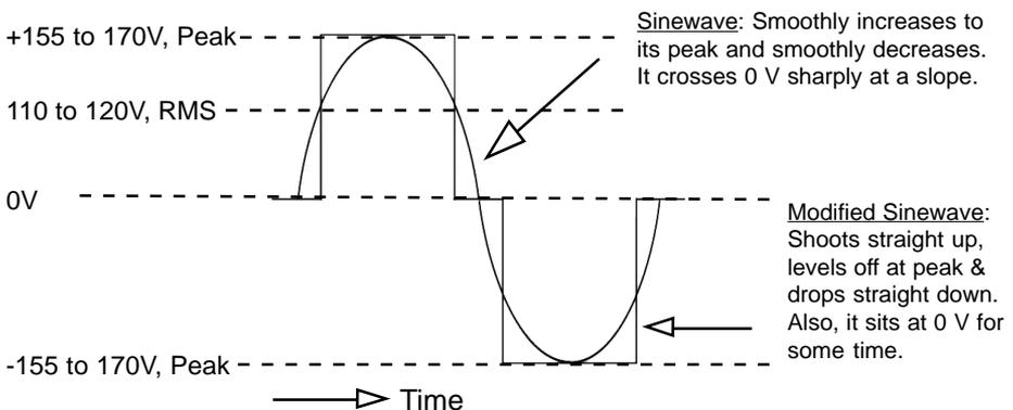
The modified sine wave produced by inverters has a root mean square (RMS) voltage of 110 to 120 volts. The majority of AC voltmeters are not calibrated to measure true RMS voltage and assume that the measured waveform will be a pure sine wave.
