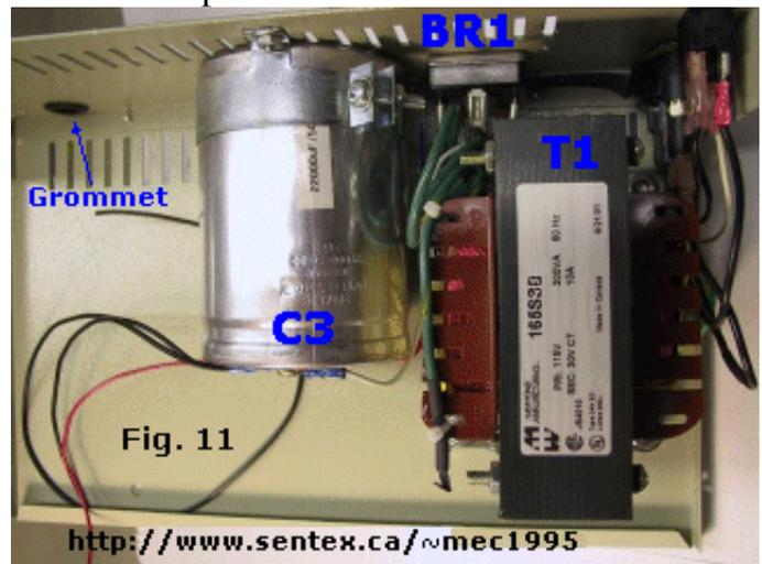
I purchased a brand new transformer, model 165S30 manufactured by Hammond. It is of the regular kind. You can get a 'low-profile', horizontal type which mounts a bit lower. Whatever model you have or buy make sure it fits your case including the large capacitor. The 30V type is only required if you need the full 10A, otherwise a 22V-28V type will do fine. A CT (Center Tap) is NOT used.
