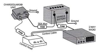
Install a 30 Amp fused lead between the battery and the Chargeguard® "BAT" lug. Install another fused jumper between the "OUT" lug and the Control Head. Connect the power lead from the radio directly to the battery. Attach the ground lead using the supplied tooth lock washer between the terminal and the vehicle chassis.
