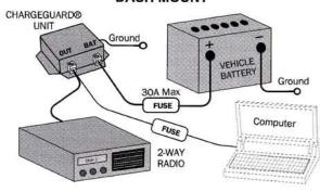
Locate the Chargeguard® unit between the vehicle battery and the Two-way Radio. Cut the power lead of the Radio leaving the fuse between the "BAT" lug and the battery. Insert the lead from the radio into the "OUT" lug and the lead from the battery into the "BAT" lug. Attach the ground lead using the supplied tooth lock washer between the terminal and the vehicle chassis.
