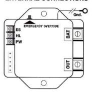
**BATT** — Connect directly to the Battery
