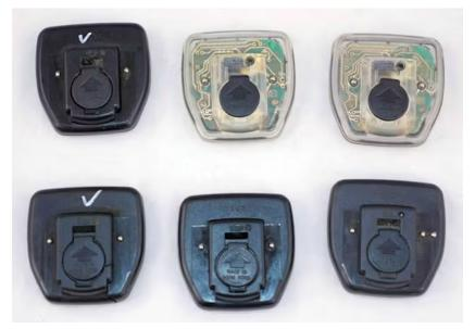
The backside of the Trek Sensor speedometer has a compartment for the battery as well as two molded-in contacts for the mounting shoe that connects to the magnetic pickup. You mount a magnet on the wheel and the speedo senses each full revolution. By programming in the circumference of the wheel in centimeters, you get a very accurate speedometer.
