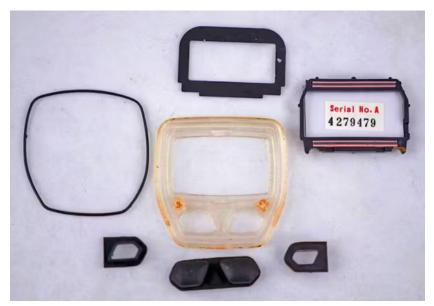
At the left is the O-ring. Above the top case-half is the black plastic placard that has the logo and model name. To the right is the LCD module, with a plastic holder and <u>zebra-strip</u> contacts to mate with the PCB. At the bottom is the rubber pushbutton surface and two black plastic retainers.
