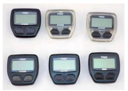
The Trek Sensor bicycle speedometer is an older model that works fine on motorcycles. They came in opaque and clear cases. The very early model was called a Trek Sonic.
