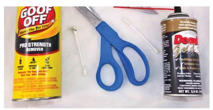
Even a simple job requires a plethora of tools. The Goof Off and DeoxIT did the work, but I needed Q-tips to scrub and apply them. An X-acto knife and scissors cut the Scotch tape. Tweezers were essential to peel the old tape off, as well as position the domes and new tape. I used the knife to pry the case-halves apart. I tried the eraser pen to clean the gold contacts, but it wasn't really needed.
