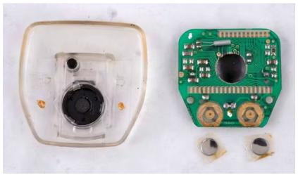
The top side of the PCB has the programming and mode switches, here removed so you can see the tape that held the spring washers to the PCB. The microcontroller is a <a href="chip-on-board">chip-on-board</a> (COB) unit, with the watch crystal at the top left along with a handful of capacitors as well as one resistor.
