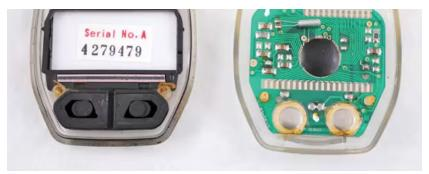
The case halves snap together. There's an O-ring on the top half that provides water resistance. The problematic switches are the two silver domes on the gold-plated pads on the PCB. You can just make out the little squares of clear tape holding the domes to the circuit board.
