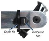
Pedal magnet on crank arm
