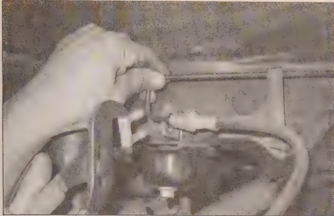
10.2 Remove the clip securing the brake line
