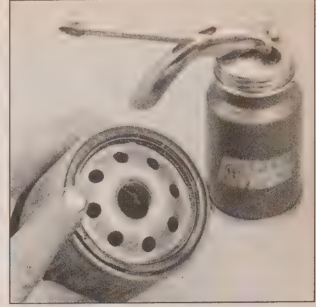
6.15 Lubricate the oil filter gasket with clean engine oil before installing the filter on the engine
