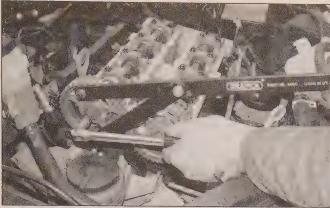
9.32 Use a sprocket holding tool while loosening the camshaft sprocket bolts
