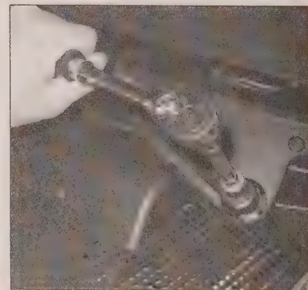
11.7a Remove each windshield wiper arm retaining nut . . .
