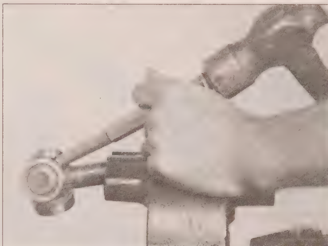
9.6a Spread the ends of the stop-ring apart and slide it towards the center of the shaft . . .
