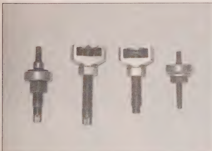
17.7 A pulley removal kit is needed to remove the power steering pulley from the 2.0L four-cylinder engine pump
