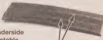
Cracks Running Parallel to "V" Portions of Belt
