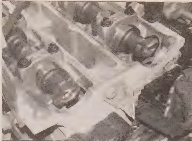
3.5a Turn the engine so that the camshaft end slots are aligned . . .
