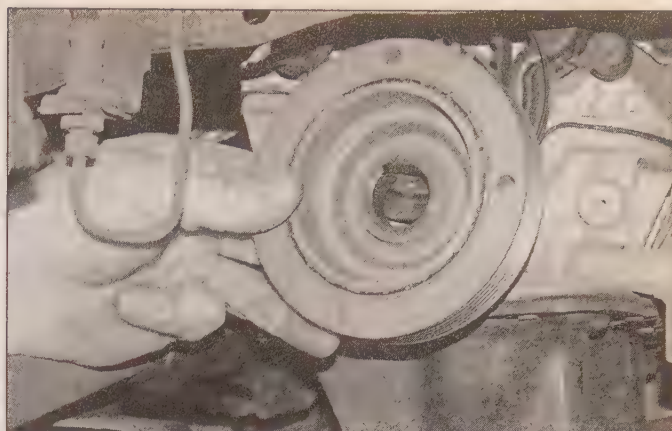
8.4b . . . and remove the crankshaft pulley
