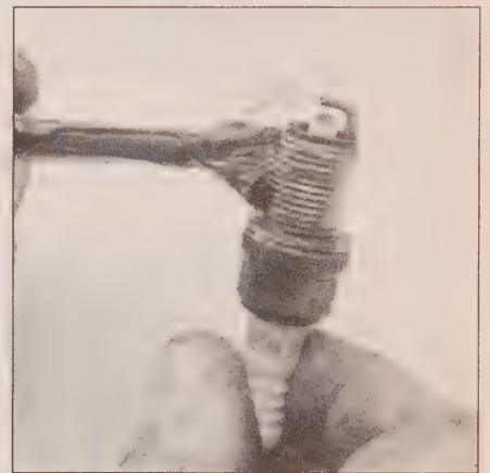
30.11a Apply a thin coat of anti-seize compound to the spark plug threads
