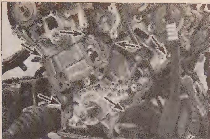
8.20 Apply a bead of RTV sealant at the locations shown
