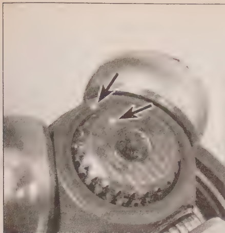
9.5 Use a center punch to place marks on the tri-pod and the driveaxle to ensure that they are properly reassembled
