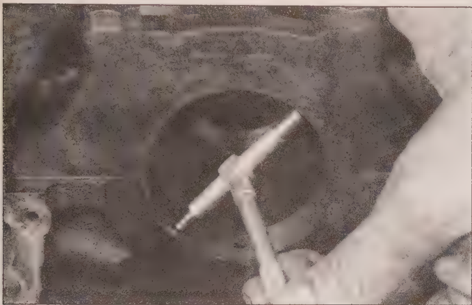
1.5 A bore gauge being used to check the main bearing bore
