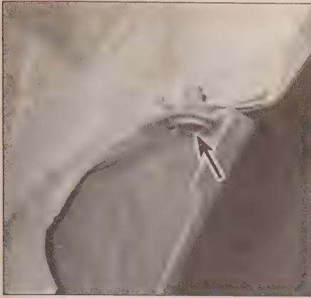
11.13 Remove the screws from the rear bumper cover and fender - one on each side of the vehicle
