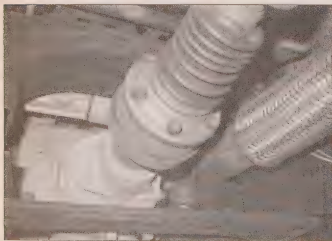
10.5 Remove the bolts securing the driveshaft to the transaxle/transfer case
