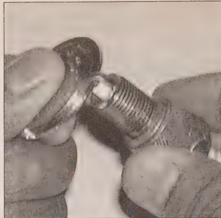
30.5a Spark plug manufacturers recommend using a tapered thickness gauge when checking the gap - slide the thin side into the gap and turn it until the gauge just fills the gap, then read the thickness on the gauge - do not force the tool into the gap or use the tapered portion to widen a gap
