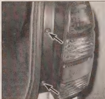
19.11a To detach the brake/tail/turn/back-up light assembly from the rear quarter panel, remove these two screws
