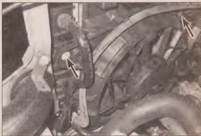
4.15 Remove the cooling fan shroud bolts - lower bolt not visible
