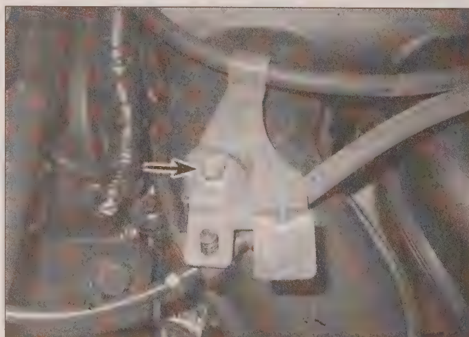
9.3 On V6 models, remove this bolt to detach the accelerator cable bracket from the intake manifold
