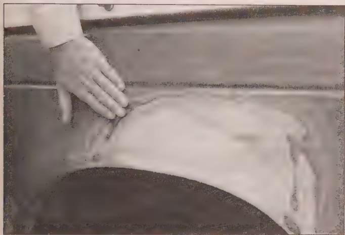
9 You shouldn't be able to feel any ridge at the transition from the filler to the bare metal or from the bare metal to the old paint. As soon as the repair is flat and uniform, remove the dust and mask off the adjacent panels or trim pieces
