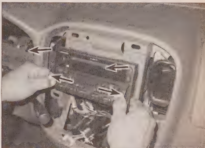
12.3 Push outward on both radio removal tools and simultaneously pull out the radio
