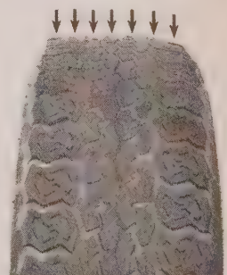
FEATHERING DUE TO MISALIGNMENT
