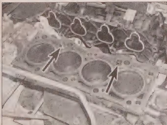
13.27 Location of the cylinder head locating dowels
