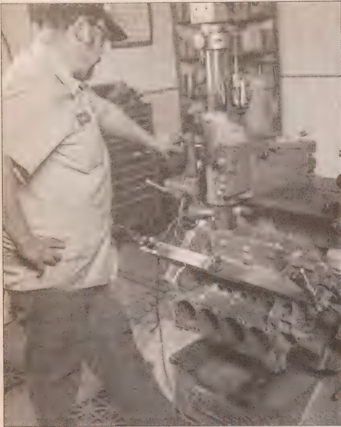
1.1 An engine block being bored. An engine rebuilder will use special machinery to recondition the cylinder bores
