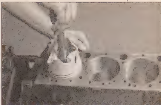
9.13 Install the piston ring into the cylinder then push it down into position using a piston so the ring will be square in the cylinder
