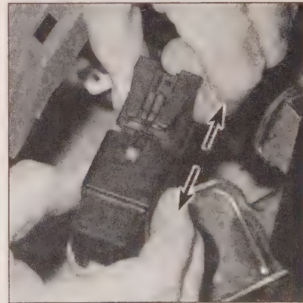
6.4c . . . and separate the connector from the turn signal/hazard flasher unit
