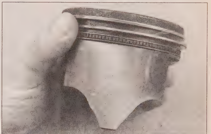
1.6 Uneven piston wear like this indicates a bent connecting rod
