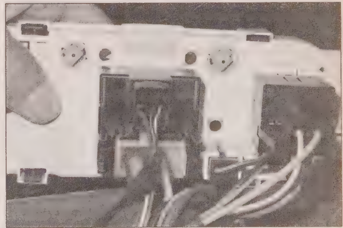
11.4b Release the tabs and disconnect the blower switch and temperature control switch connectors
