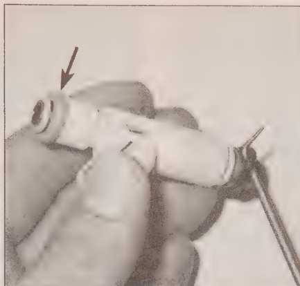
14.22 Remove the old O-rings from each injector and discard them; always install new O-rings when installing the injectors (V6 models)
