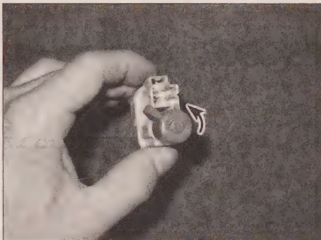
13.2 Rotate the knob counterclockwise until it stops to unlock the switch
