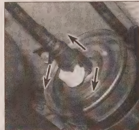
4.3e . . . then grasp the coupling and line and pull it straight off the pipe on the filter (this type of R-clip coupling is also referred to as a "horseshoe clip" coupling because of the shape of the clip)
