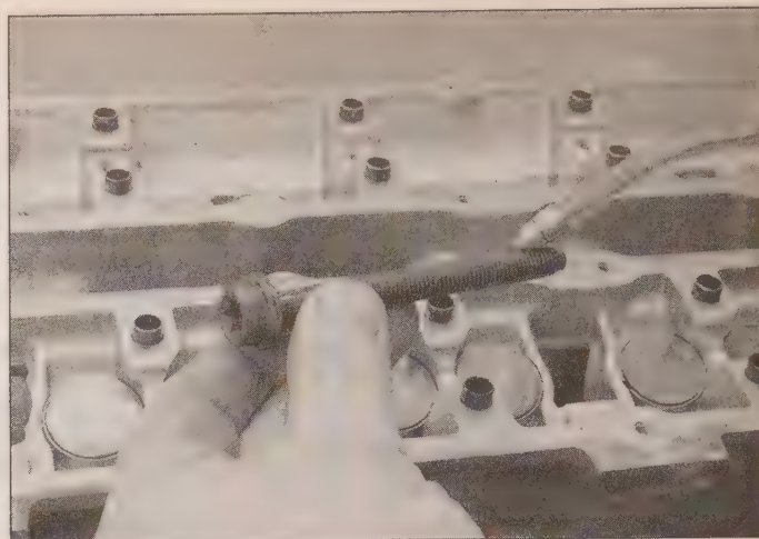
13.34 Apply a light coat of oil to the cylinder head bolt threads
