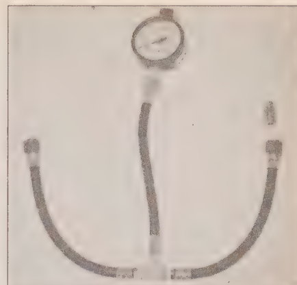
3.3c A typical fuel pressure gauge setup suitable for checking the fuel pressure on four-cylinder models; these models don't have a Schrader valve test port on the fuel rail, so you'll have to disconnect the fuel supply line at the fuel rail (or at some other fuel supply line connection in the engine compartment) and tee into it
