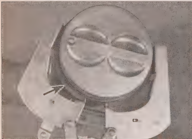
9.22 Use a piston ring installation tool to install the number 2 and the number 1 (top) rings - be sure the directional mark on the piston ring(s) is facing toward the top of the piston
