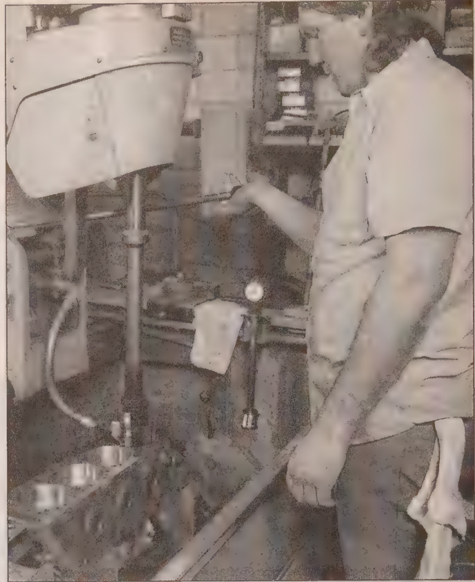
1.2 If the cylinders are bored, the machine shop will normally hone the engine on a machine like this
