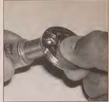
30.5b To change the gap, bend the side electrode only, using the adjuster hole in the tool, and be very careful not to crack or chip the porcelain insulator surrounding the center electrode
