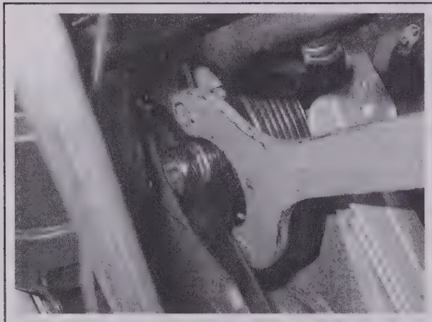
17.12 With the pulley secured, remove the pulley mounting nut
