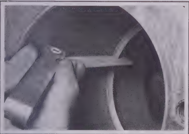
9.14 With the ring square in the cylinder, measure the ring end gap with a feeler gauge
