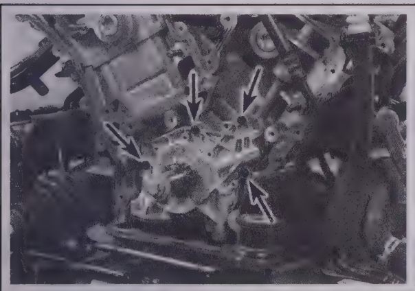
13.3 Remove the oil pump retaining bolts and pull the oil pump off the crankshaft
