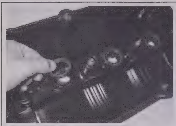
4.8b Remove and discard the spark plug tube seals from the valve cover
