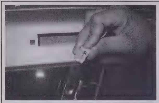
19.6b Pull out the high-mount brake light assembly and disconnect the electrical connector
