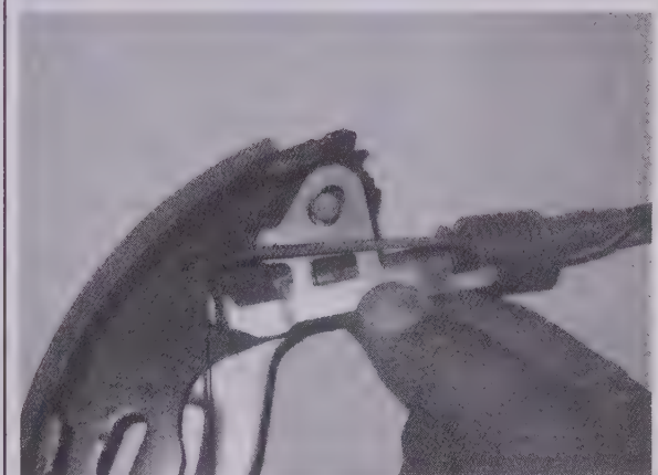
6.6g On the rear shoe, remove the self-adjust lever . . .
