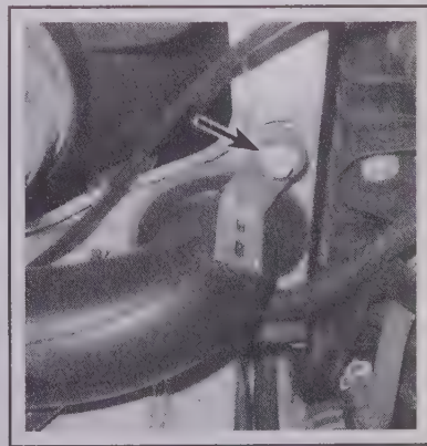
8.10 To detach the fresh air inlet duct from the vehicle body, remove this bolt
