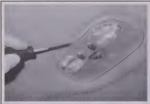
19.21 To remove the interior/map reading light lens, carefully pry it off with a small screwdriver inserted into this slot, which is provided for this purpose (prying off the lens elsewhere might damage or scratch the housing)
