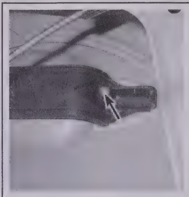
17.5 Remove this door latch assembly screw
