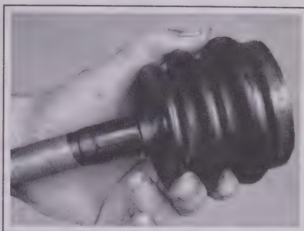
9.11 Wrap the splined area of the axle shaft with tape to prevent damage to the boot(s) when installing it
