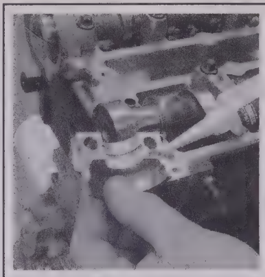
12.21 Apply sealant to each of the bearing caps at the timing belt end
