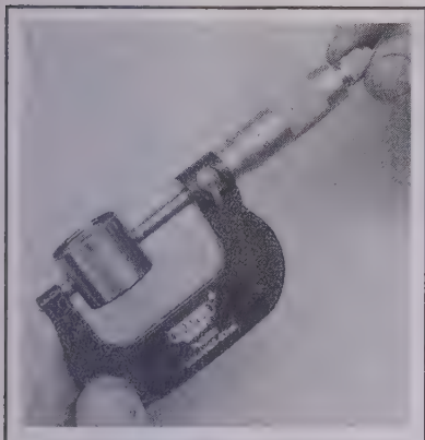
12.8 Measure the cam follower outside diameter at several points
