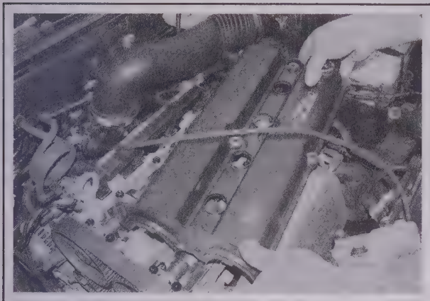
4.8b . . . lift off the valve cover from the cylinder head
