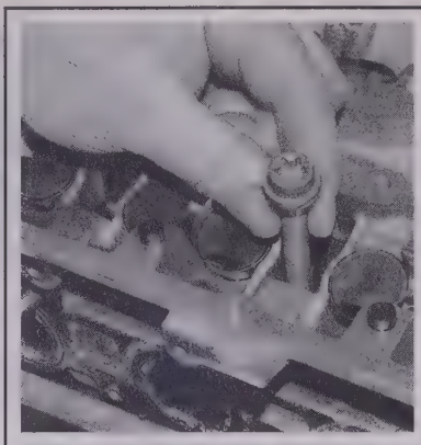
13.19 Remove the cylinder head bolts - note the head bolt uses a Torx socket
