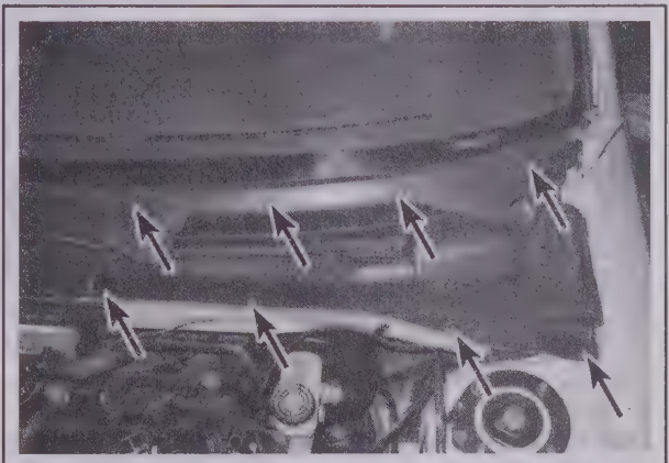
14.2b Location of the left cowl cover fasteners
