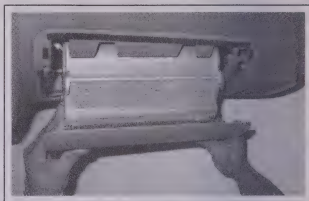
25.18 Pull the trim cover and the airbag from the dash as a single assembly. Be sure to keep your body positioned to the side of the airbag
