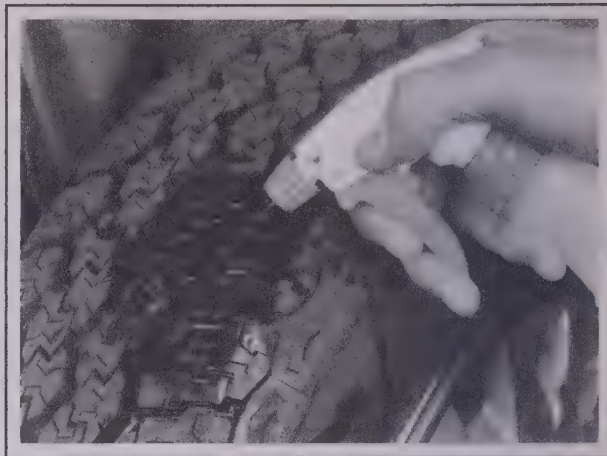
5.4b If the valve core is tight, raise the corner of the vehicle with the low tire and spray a soapy water solution onto the tread as the tire is turned slowly - slow leaks will cause small bubbles to appear
