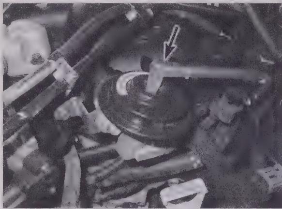
21.26 Disconnect the vacuum line from the EGR valve (V6 models)
