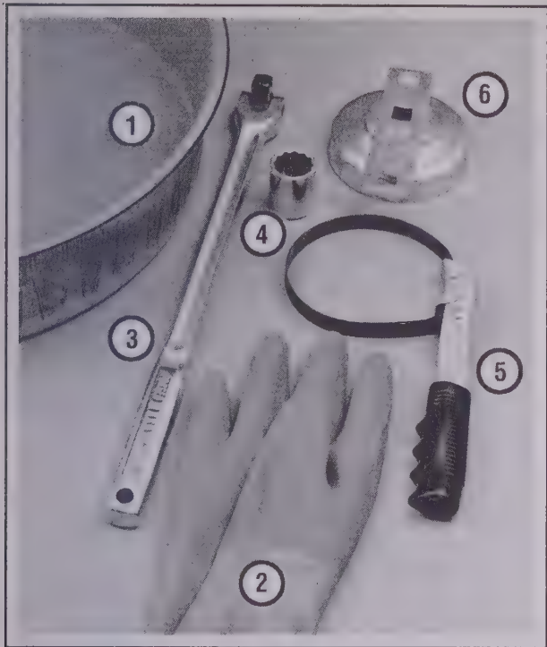
6.2 These tools are required when changing the engine oil and filter
