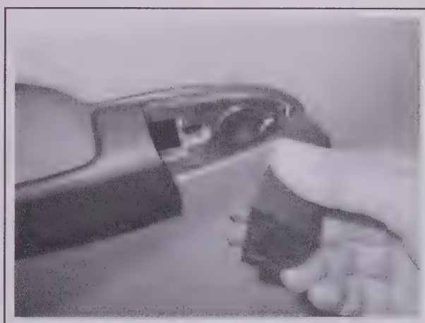
17.18 Remove the cover from the rear door handle
