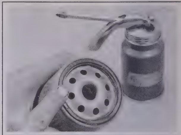
6.15 Lubricate the oil filter gasket with clean engine oil before installing the filter on the engine
