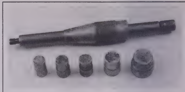
6.4 A clutch alignment tool is necessary if you plan to install a rebuilt engine mated to a manual transaxle
