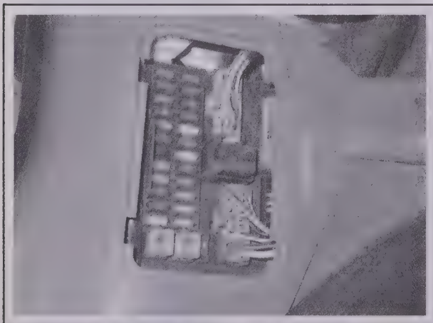
3.1c The passenger compartment fuse/relay box is located either in the left kick panel as shown, or on the right-hand side of the center console. It contains fuses and relays
