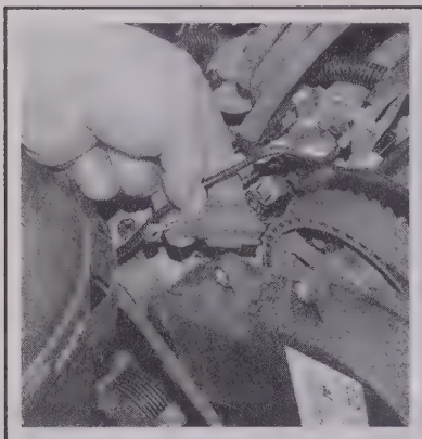
9.19a Disconnect the harness connector next to the upper timing belt cover
