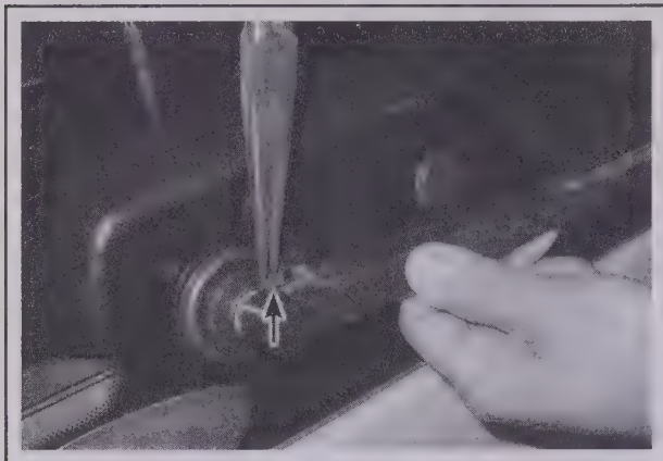
11.16 To detach the rear window wiper arm from the shaft, pull this locking tab straight up with a pair of needle-nose pliers, then pull the wiper arm straight off the shaft
