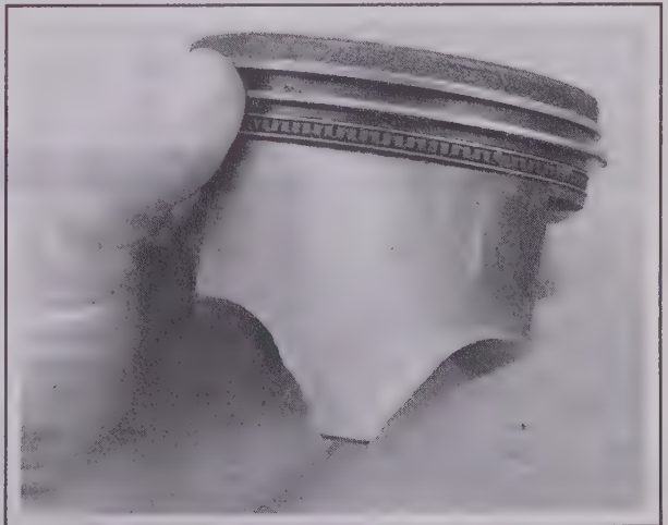
1.6 Uneven piston wear like this indicates a bent connecting rod
