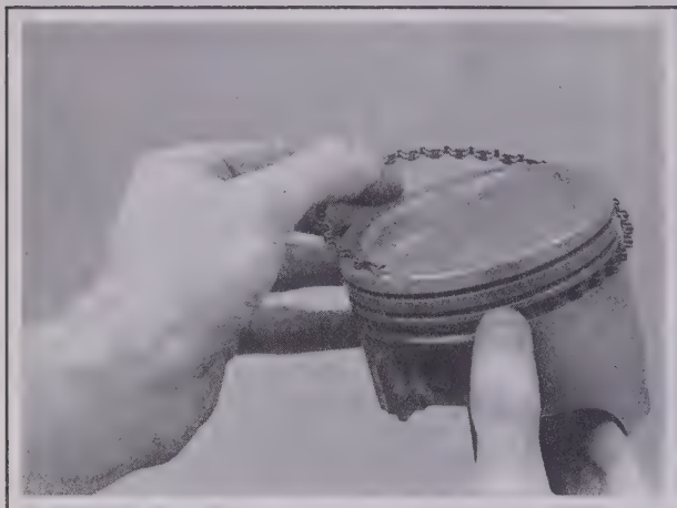
9.19a Installing the spacer/expander in the oil ring groove
