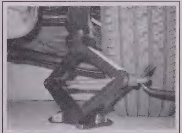
Rear jacking location (place the jack head under the protrusion on the trailing arm)
