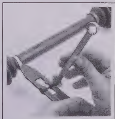
9.17c To install band-type clamps you'll need a special tool; install the band with its end pointing in the direction of axle rotation and tighten it securely, then pivot the tool up 90-degrees and tap the center of the clip with a center punch . . .
