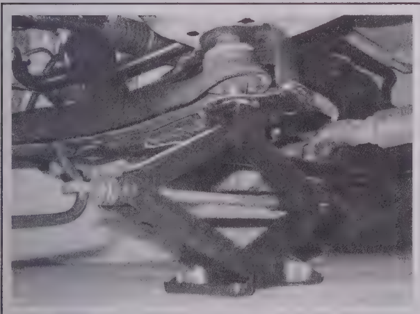
Front jacking location (place the jack head under the control arm rear mounting bolt)
