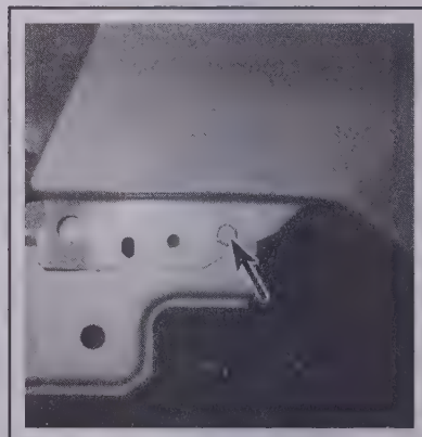
12.10a Location of the fender corner bolt
