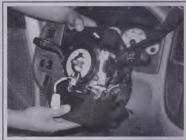
25.2b Separate the upper and lower steering column covers (steering wheel removed for clarity)
