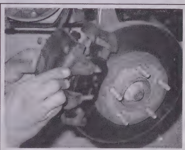
3.6m Install the caliper and tighten the caliper mounting bolts to the torque listed in this Chapter's Specifications
