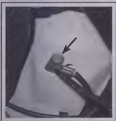
4.4a To detach the ground cable from the left fender, remove this bolt
