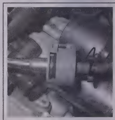
4.10b . . . close the clamshell halves of the tool around the coupling . . .
