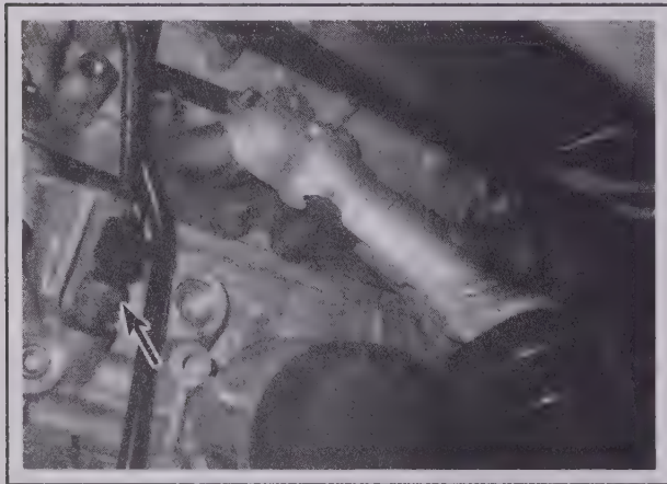
2.2b On V6 engines the oil pressure sending unit is located on the front of the engine block behind the air conditioning compressor
