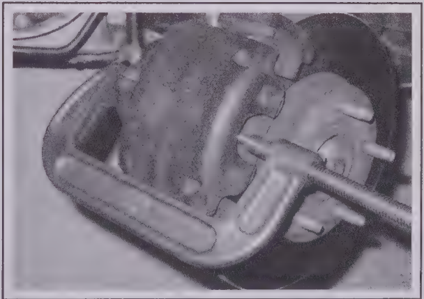
3.5 Before removing the caliper, be sure to depress the piston into the bottom of its bore in the caliper with a large C-clamp to make room for the new pads
