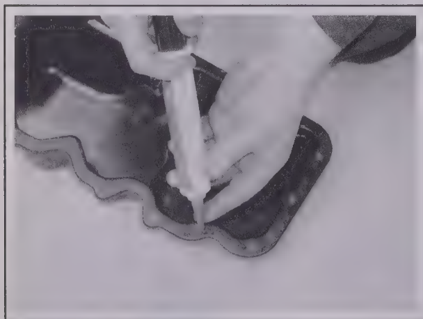
14.7 Apply a bead of sealant to the oil pan flange, inboard of the bolt holes
