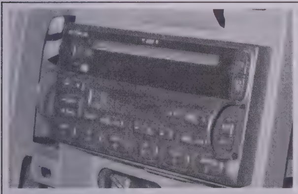
12.2b Insert the special radio removal tools into the holes at each end of the radio as shown, then push them in until you feel the internal clips release
