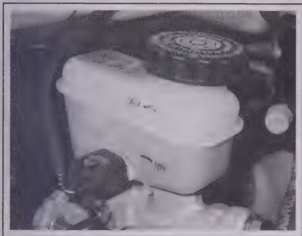
4.15 The brake fluid level should be kept between the MIN and MAX marks on the translucent plastic reservoir; the same reservoir contains the clutch fluid and is connected to the clutch master cylinder by a hose
