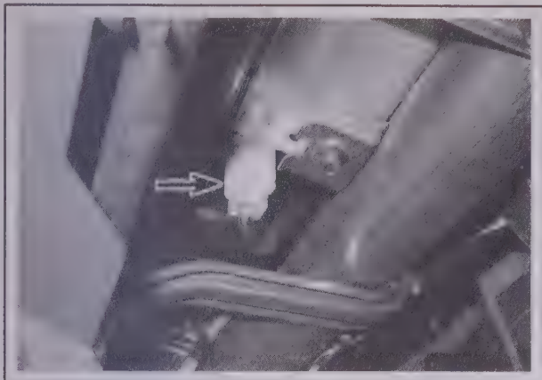
25.11 The electrical connector for the passenger's side airbag is located above the glove box recess, to the left of the airbag module (glove box removed for clarity)
