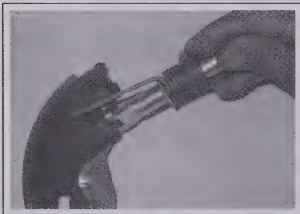
6.6n Insert the adjuster screw into its slot on the rear shoe and attach the return spring
