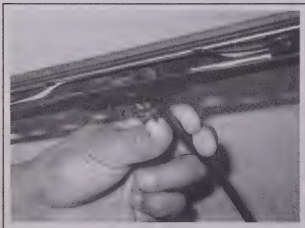
7.4a To release the blade holder, push the release pin . . .
