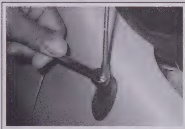
13.1 Unscrew the antenna mast with a 10 mm wrench
