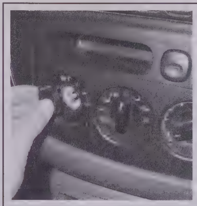
24.11 Remove the climate control knobs from the control assembly
