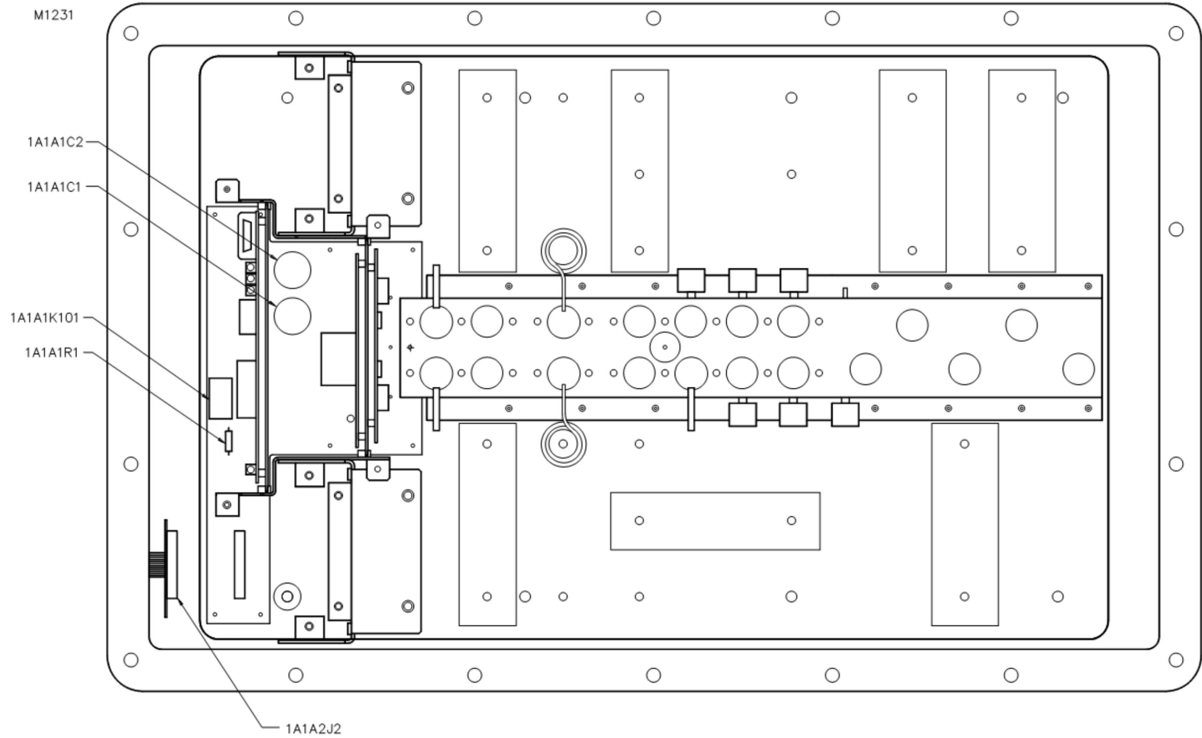
Figure 5.7-3. Non-Chassis Component Locations
