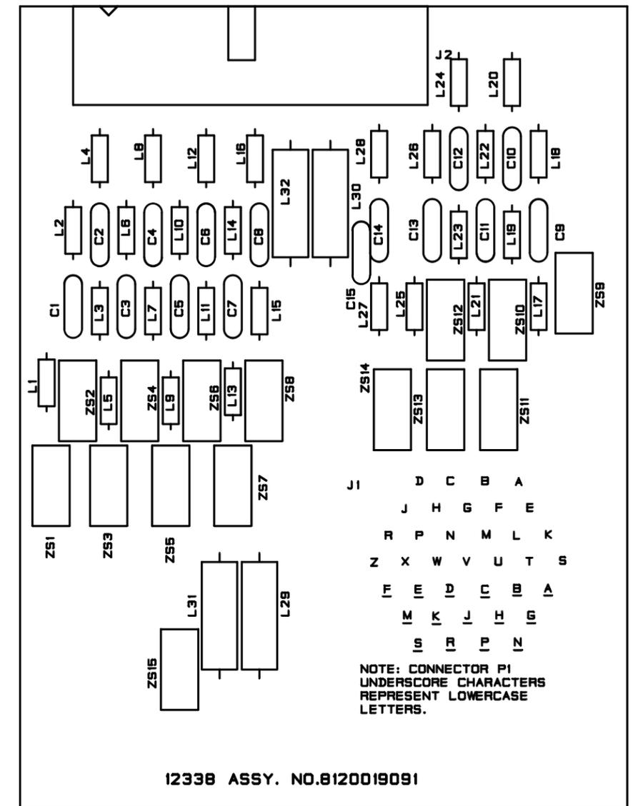
Figure 5.7-6. PC Assembly, Input Connector, 1A1A2
