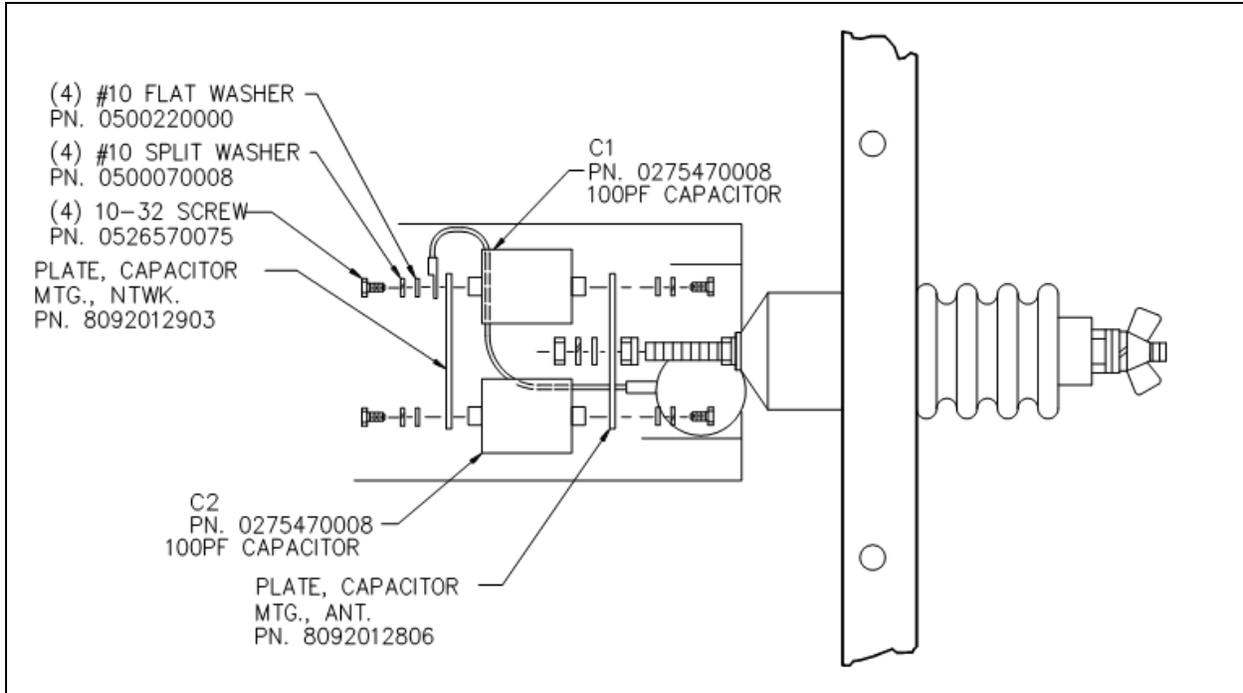
**Figure 2.11-6. Long-Wire Adapter Kit (1A1A5) 81200909003 Installation Configured for Long-Wire Operation**
