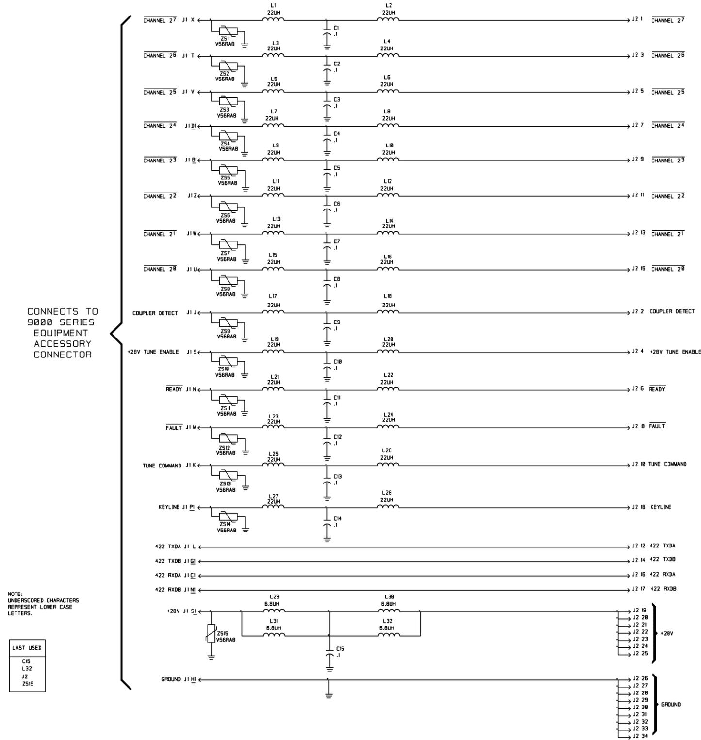
Figure 5.7-6. PC Assembly, Input Connector, 1A1A2
