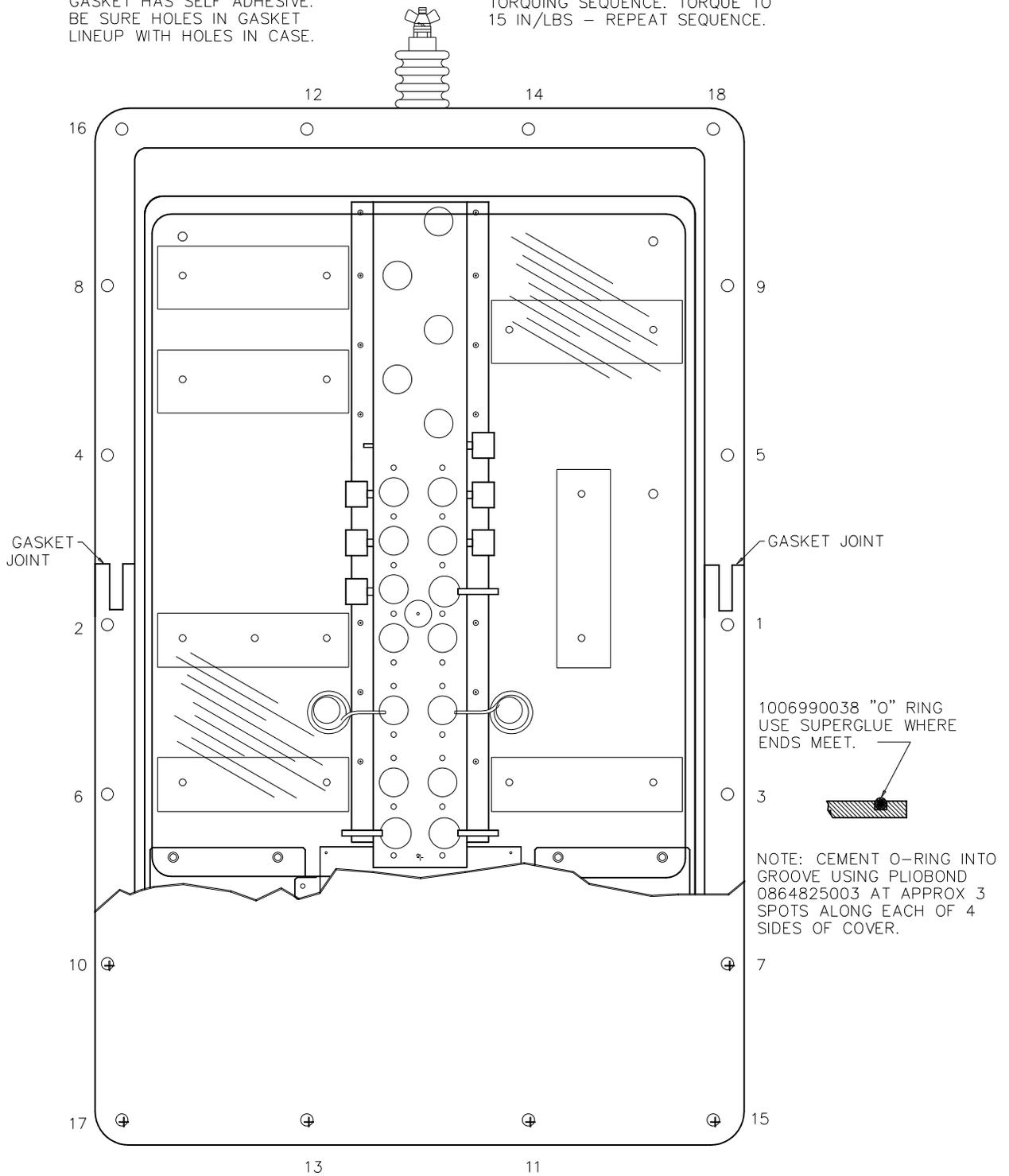
**Figure 5.2-1. Gasket Installation and Torque Sequence**
