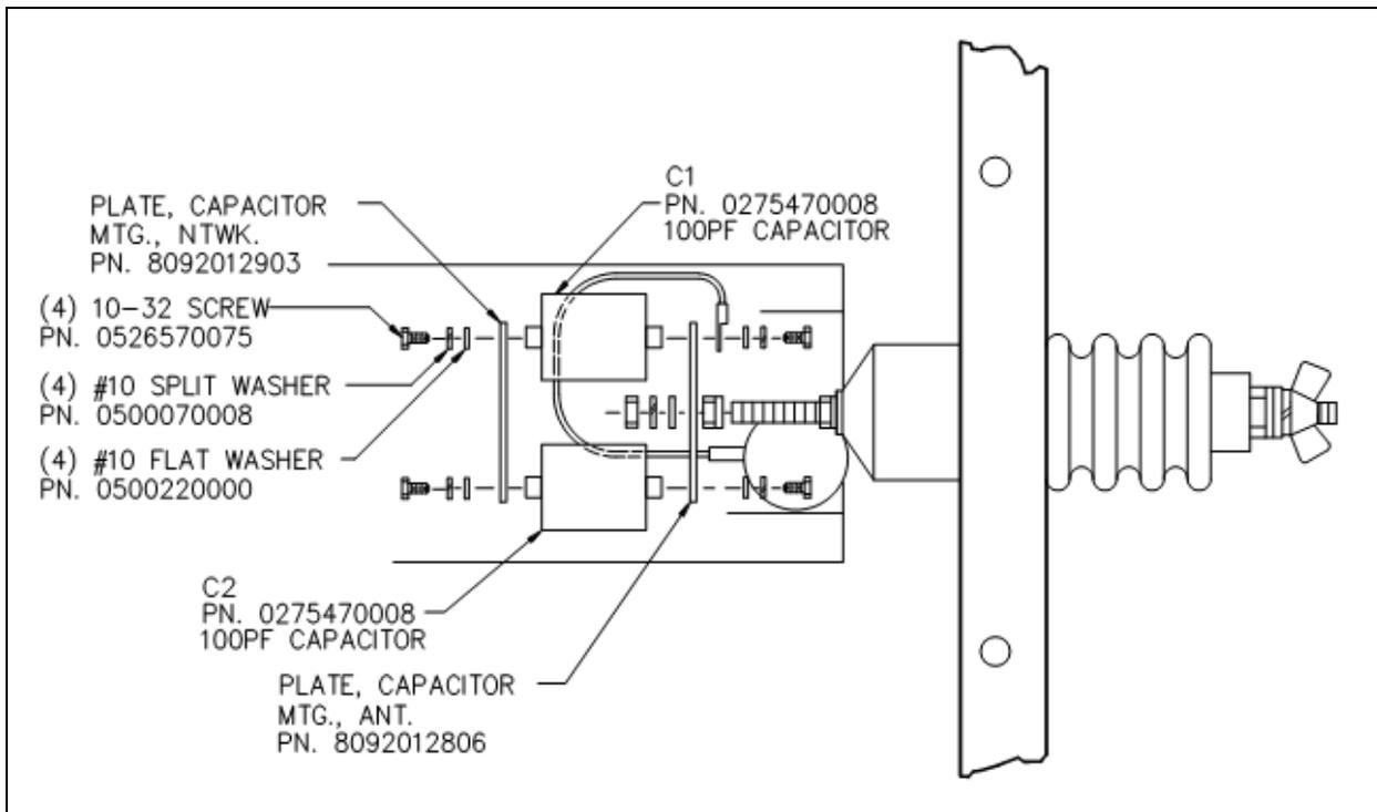
**Figure 2.11-7. Long-Wire Adapter Kit (1A1A5) 81200909003 Installation Configured for Whip Wire Operation**
