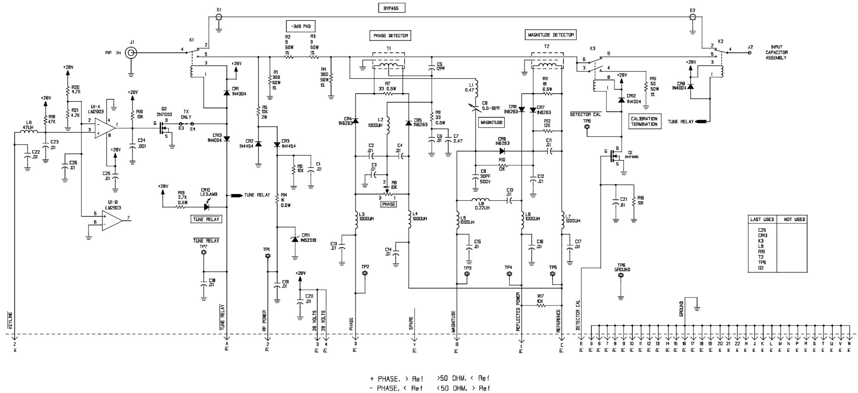
Figure 5.7-8. PC Assembly, RF Detector, 1A1A4A1
