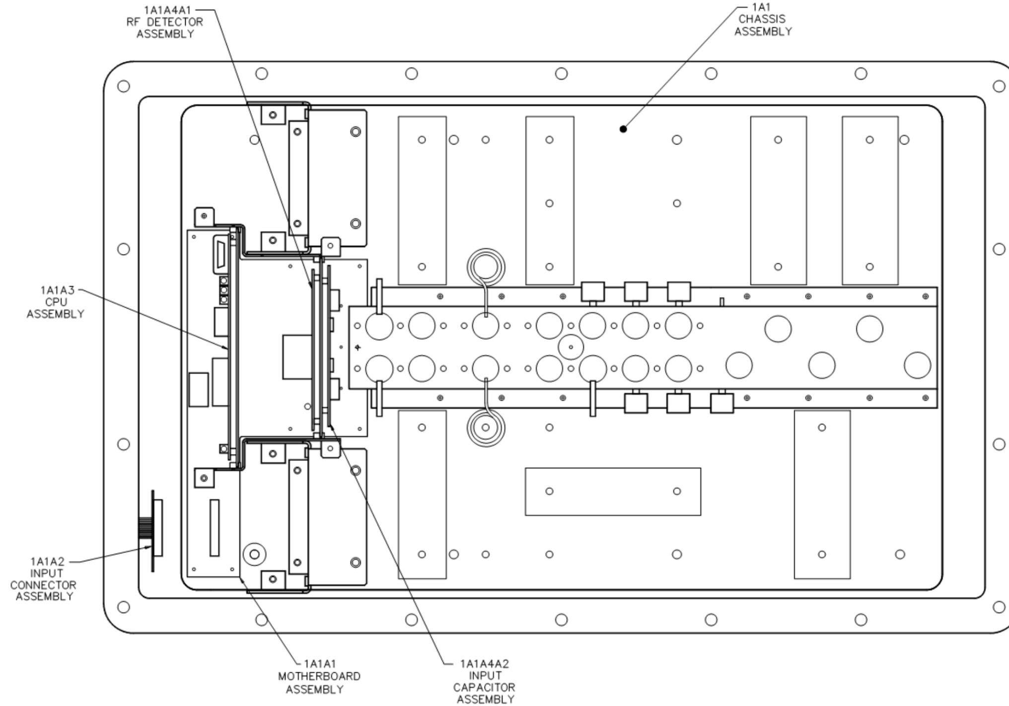
Figure 5.7-1 CU-9150 Assembly Locations
