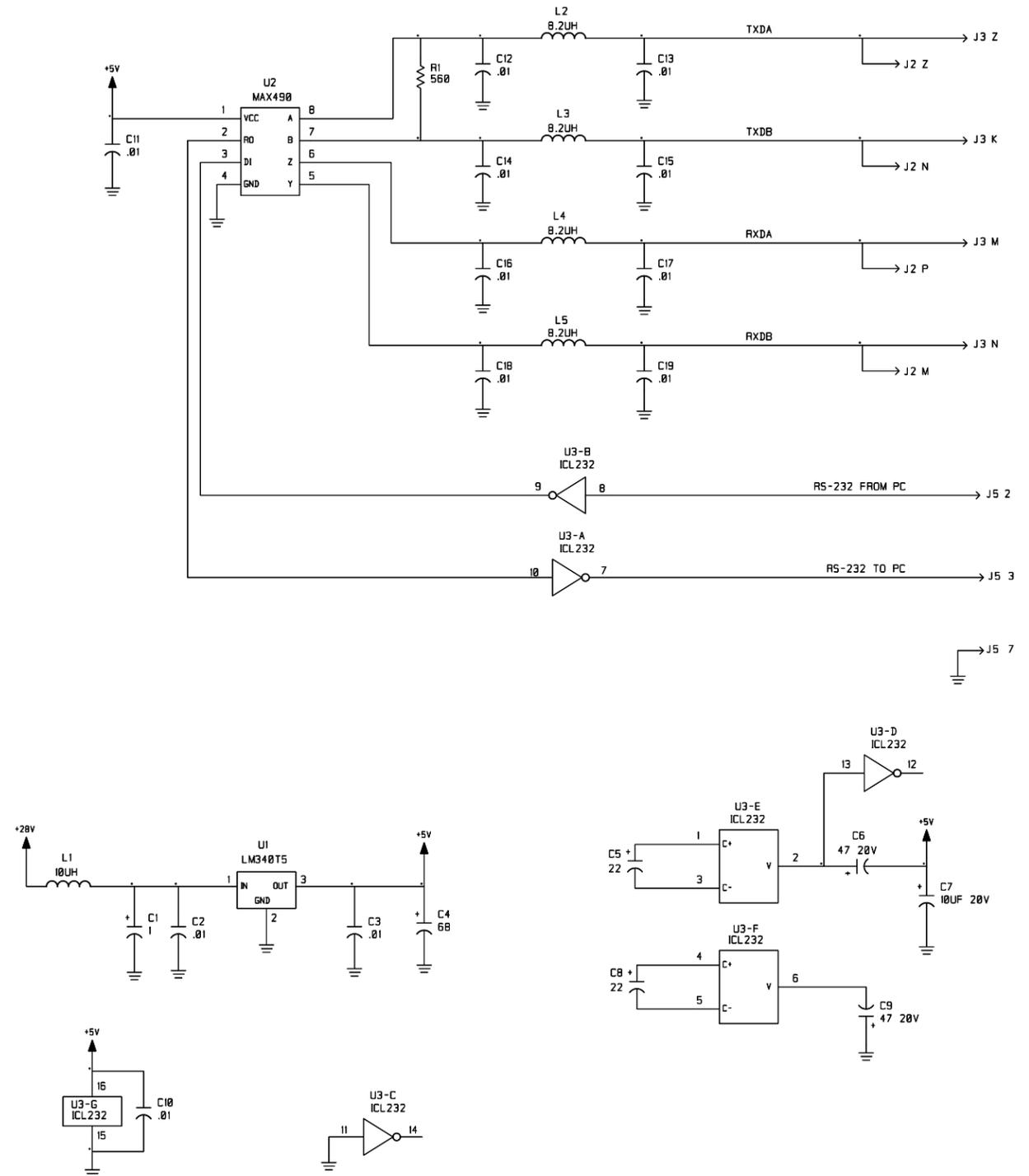
**Figure 6.1-2. PC Assembly, Serial Breakout Board**
