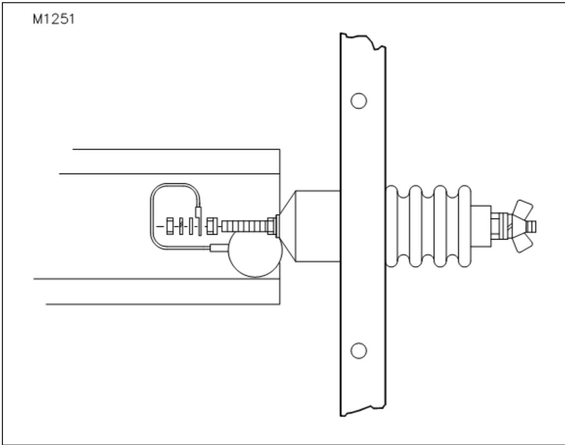
**Figure 2.11-8. Assembly/Disassembly of Antenna Output Lead (Long-Wire Adapter Kit Not Installed)**
