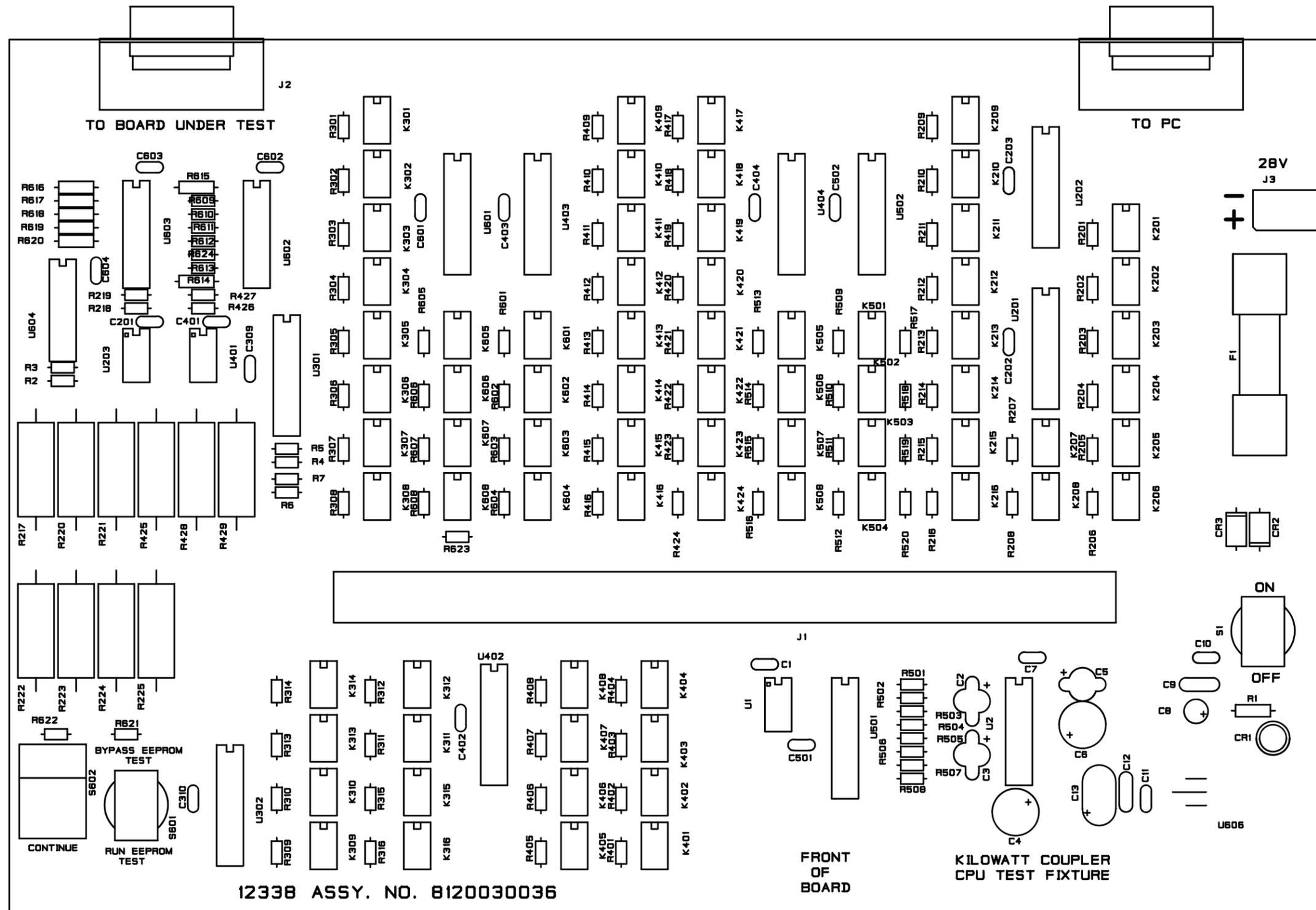
Figure 6.1-1. PC Assembly, Test Fixture, CU-9150 CPU
