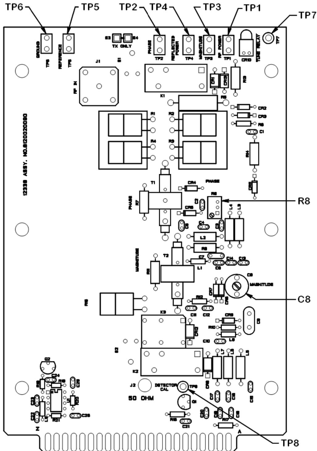
Figure 5.5-1. 1A1A4A1 RF Detector Alignment Adjustment Locations
