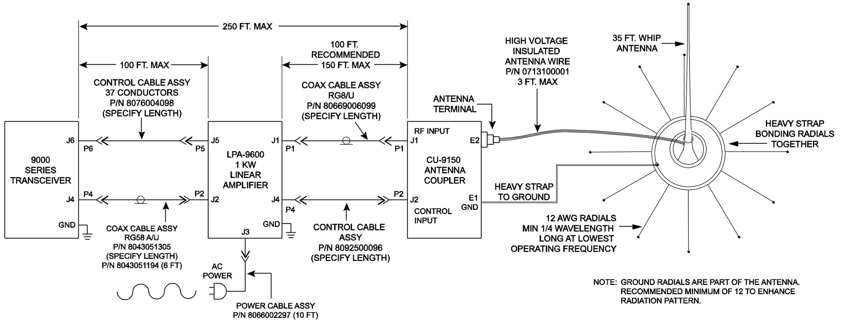
Figure 2.11-3. LPA-9600 with CU-9150, 35-Foot Antenna (Roof Top Installation)
