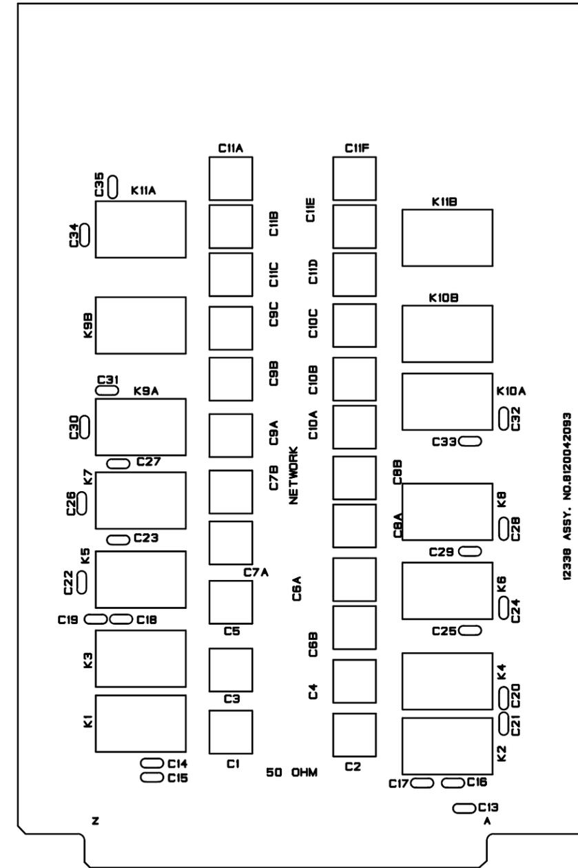
Figure 5.7-9. PC Assembly, PC Assembly, Input Capacitor, 1A1A4A2
