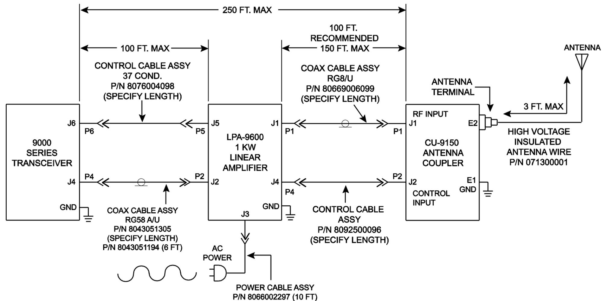
Figure 2.11-4. LPA-9600 with CU-9150, Non-Resonant Antenna
