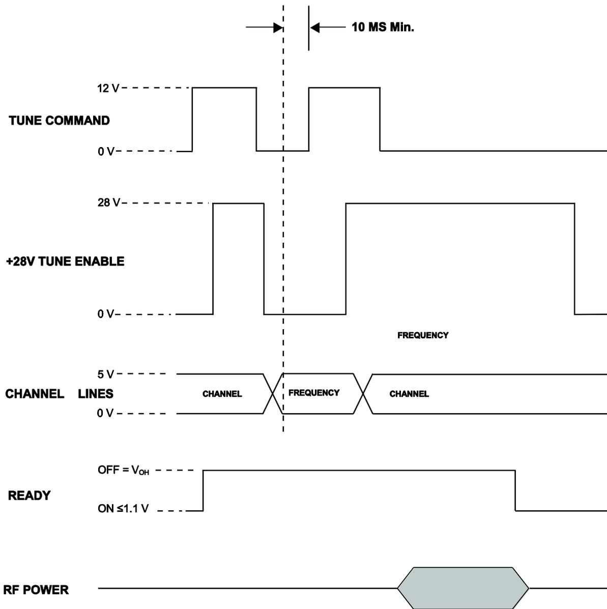
Figure 4.9-1. Coupler Interface Timing
