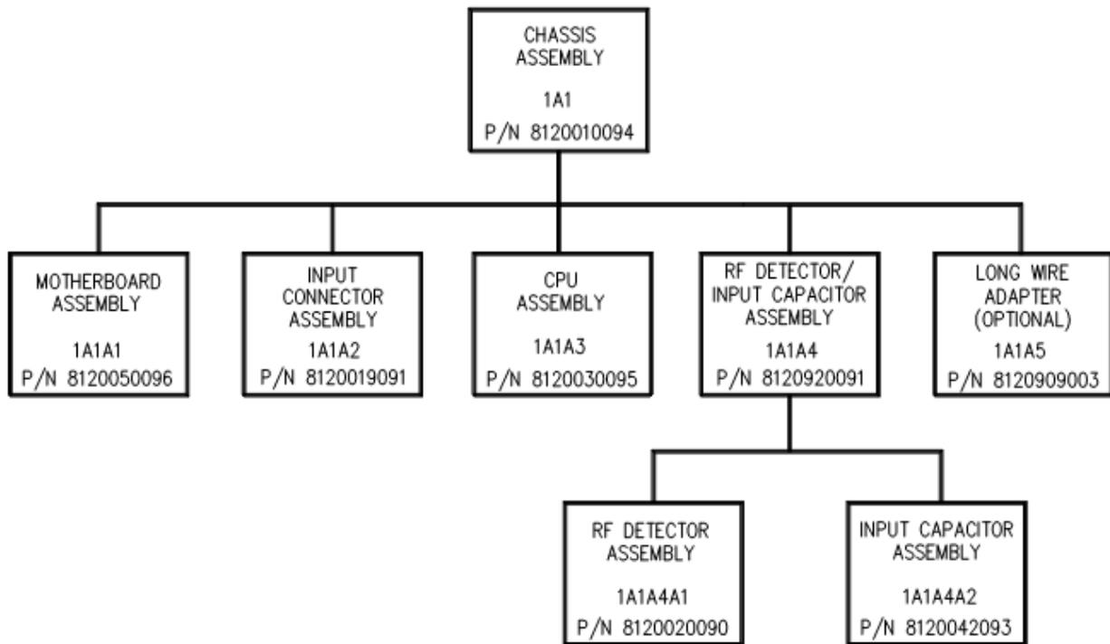
Figure 4.9-2. CU-9150 Assembly Tree
