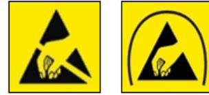
Electrostatic Discharge (ESD) can severely damage sensitive components located on printed circuit cards. Electrostatic discharge measurements as high as 35,000 volts, can occur from walking across a carpet.
