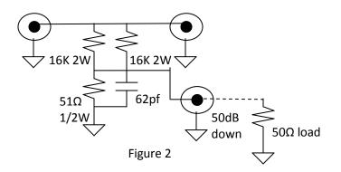
You'll also note the 62pf capacitor. I found that the 51 ohm resistor is slightly more inductive than the two parallel 16K resistors, resulting in peaking of the detected power as the frequency was increased. The 62pf capacitor helps compensate this at the higher frequencies.
