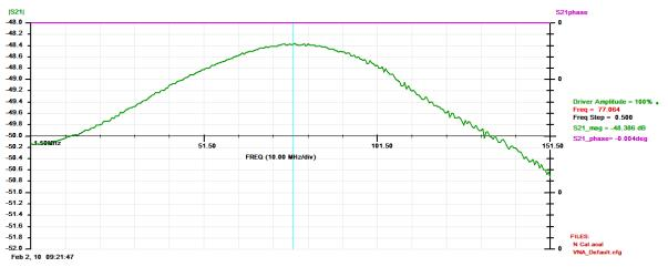
Figure 3 – Swept coupling response from 1.5-150 MHz
