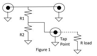
For my 50dB tap, I wanted to use commonly available resistors. It turns out that 8K ohms and 25 ohms will give you the desired 50dB tap point:
