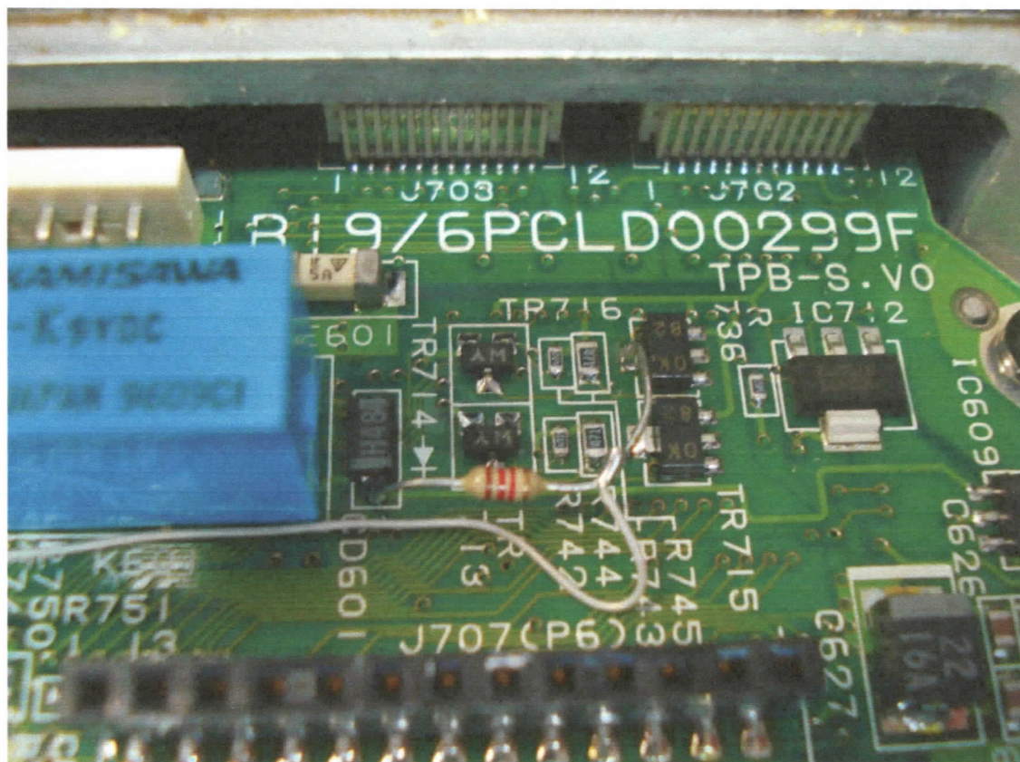
Another view of wire connection to resistor top side
