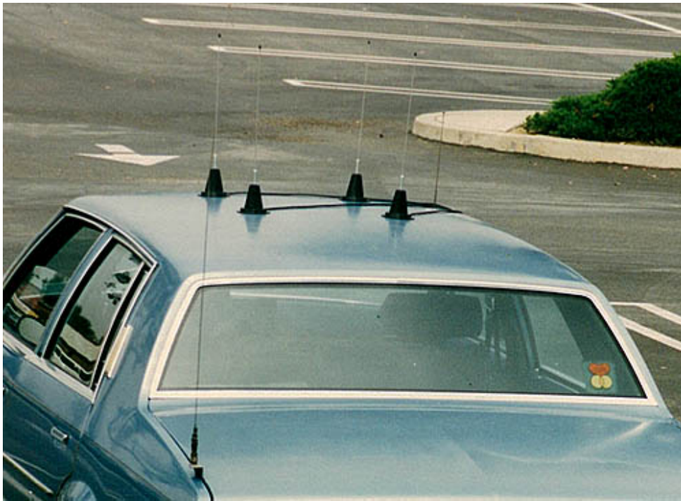
Photo 4. Magnetic-mount doppler whips can be placed quickly on any vehicle with a ferrous metal top and moved about to cover a wide range of frequencies.
