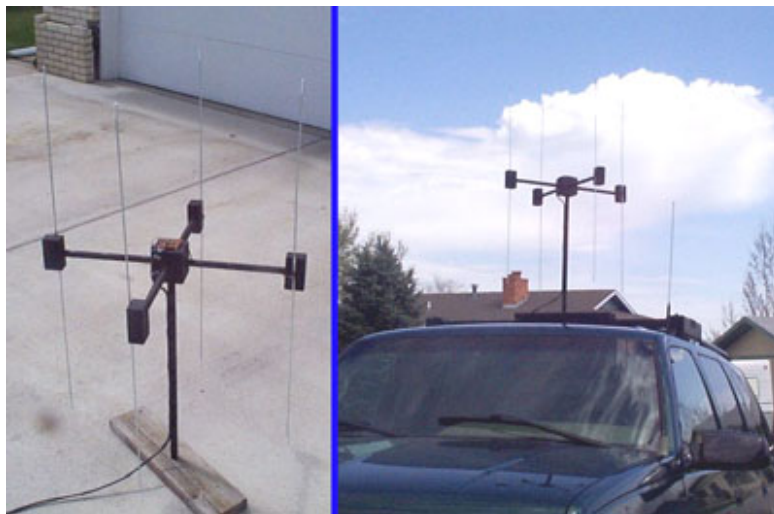
Photo 9. Vincent Fiscus KB7ADL built his two-meter Roanoke Doppler antenna using dipoles instead of quarter-wavelength whips. He reports that weak-signal and multipath performance is better. (Photos by KB7ADL)
