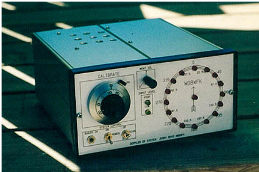
Photo 1 (left). This Roanoke Doppler display box was built by Jerry Boyd WB8WFK of Albuquerque, NM. Note the 10-turn potentiometer and large dial for the calibration control. This allows him to log settings for each band. (Photo by WB8WFK)
