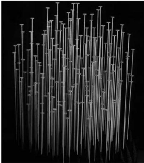
**FIGURE 1-23** Volumetric array antenna with randomly distributed loop elements: Crow's nest antenna by FGAN e.V., Wachtberg, Germany<sup>20</sup> (Courtesy of FGAN e.V., Wachtberg, Germany)
