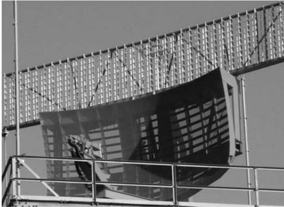
**FIGURE 43-10** Open-array SSR antenna. The ladder-like top section makes up the SSR directional antenna.
