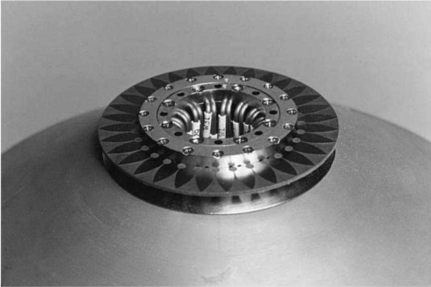
**FIGURE 22-18** Circular array (Courtesy of Anaren Corporation)
