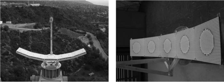
**FIGURE 35-24** Piece-wise flat reflectarray for space application
