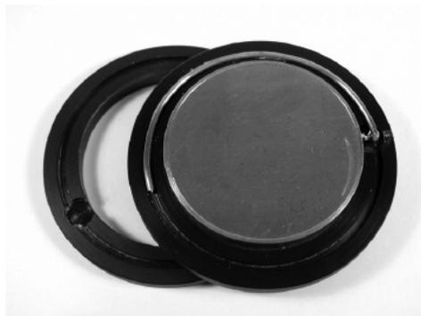
**FIGURE 38-11** Circumference antenna on a pacemaker model (after A. Johansson,<sup>169</sup> Figure 5-3)
