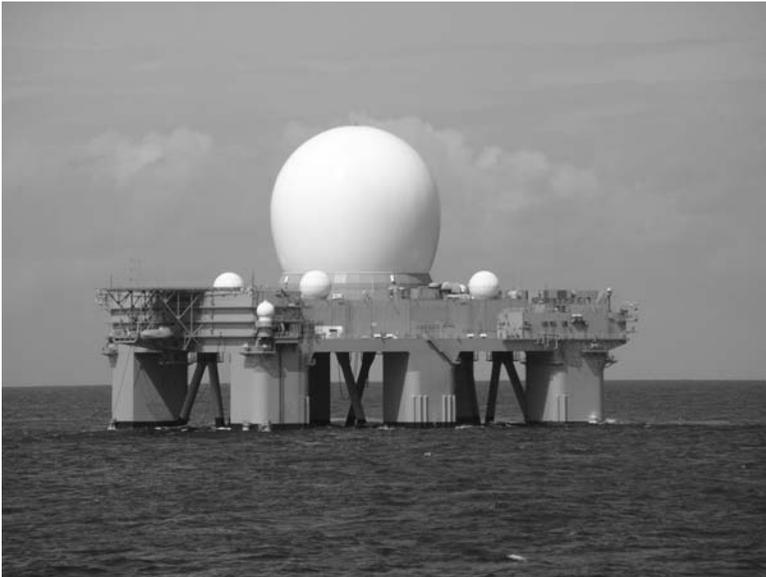
(b) Radomes for sea-based radar and communication antennas
