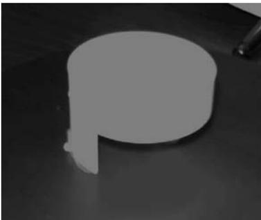
**FIGURE 17-14** Shaped DRA: DCS-WLAN bands
