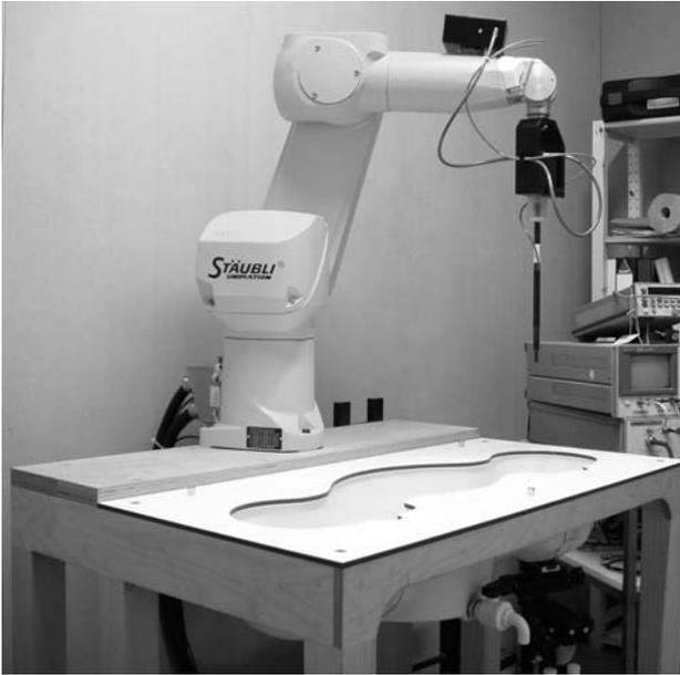
FIGURE 36-14 DASY 4 SAR measurement system by SPEAG
