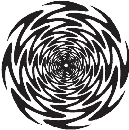
FIGURE 13-75 An eight-arm self-complementary sinuous antenna
