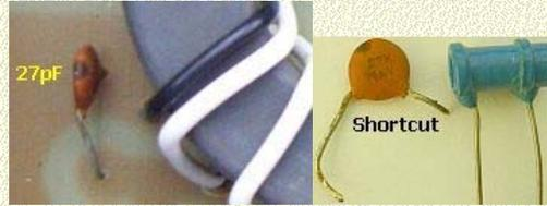
I replaced a shortcut 27 pF cap with 4 × ceramic tube caps in series/parallel.
