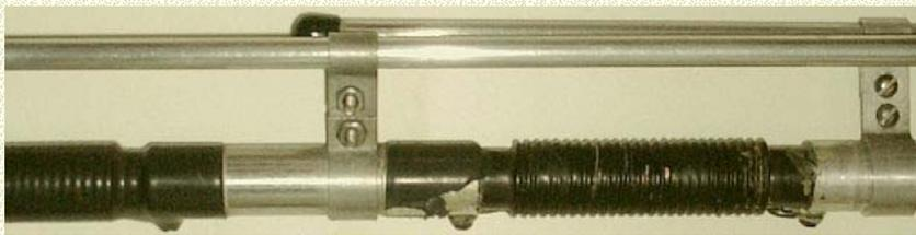
Water got inside a trap due to cracked heath shrink tubing.
