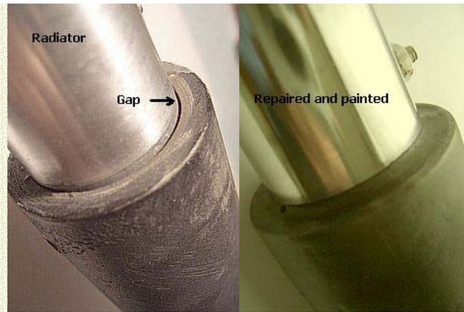
The antenna wobbled due to the gap caused by evaporation of the polyester. The tube was removed, the inside of the insulator applied with layers of 2 component polyester resin until a minimum variation of fit of the tube. Then I sanded the insulator for a perfect cylindrically curved shape and applied the last layer and placed the antenna back in the insulator. In fact the insulator was restructured to its original diameter.
