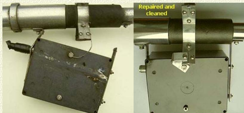
Due to the gap the antenna wobbled and one of the straps was broken.
