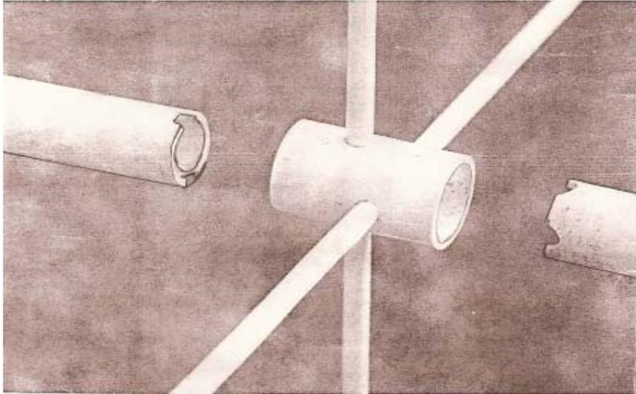
Figure 4.7 The Collapsible version boom is knotted for proper alignment
