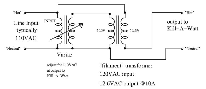
The Variac does not need to be rated for more than about 100 watts, as it's only used to drive the filament transformer primary. Of course, if you have a great big Variac that can handle 1100 Watts, then just use that, and you can skip the filament transformer. In that case, just hook the Kill-A-Watt that you're calibrating to the output of your huge Variac.
