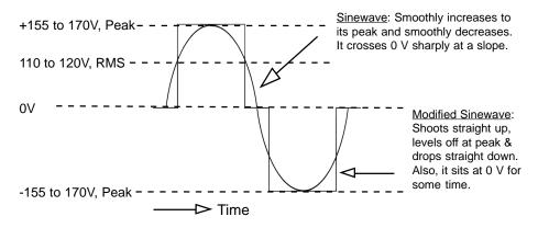
The modified sine wave produced by inverters has a root mean square (RMS) voltage of 110 to 120 volts. The majority of AC voltmeters are not calibrated to measure true RMS voltage and assume that the measured waveform will be a pure sine wave.
