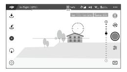
After confirming the selection, the aircraft will fly in the direction marked by the "GO" icon. The aircraft will automatically adjust its speed when it senses an obstacle out in front or if it is flying too close to the ground. However, this feature should not be relied upon for navigation between obstacles.
