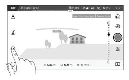
3. Tap on the subject you want to track then tap to confirm your selection. If the subject is not automatically recognized, drag a box around it. The box will turn green when tracking is in progress. If the box turns red, the object could not be identified and you should try again.
