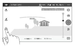
3. Tap once on the target and wait for the "GO" icon to appear. Tap the "GO" icon to confirm the selection and the aircraft will fly to the target automatically. There will be a prompt if the target cannot be reached. If this is the case, select another target and try again.
