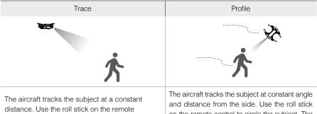
The aircraft tracks the subject at a constant distance. Use the roll stick on the remote controller or the slider in DJI GO 4 to circle the subject.
