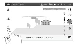
3. Tap once on the target and wait for the "GO" icon to appear. Tap the "GO" icon to confirm the selection and the aircraft will fly in that direction automatically.
