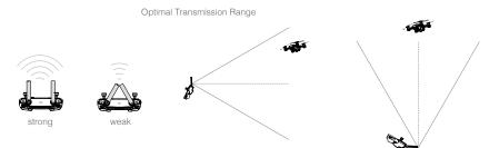
Ensure the aircraft is flying within the optimal transmission zone. To maintain optimal transmission performance, adjust the remote controller and antennas according to the above diagram.
