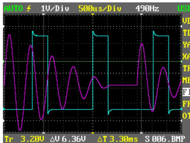
The cyan square wave is a trace of the live input signal and the purple waveform is a static reference waveform.
